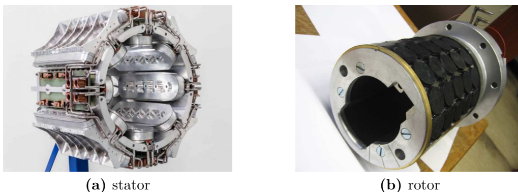
Figure 2.23. Utilisation of superconductors in electric motors as: (a) stator coils [184]; (b) superconducting bulks on rotor [26]
