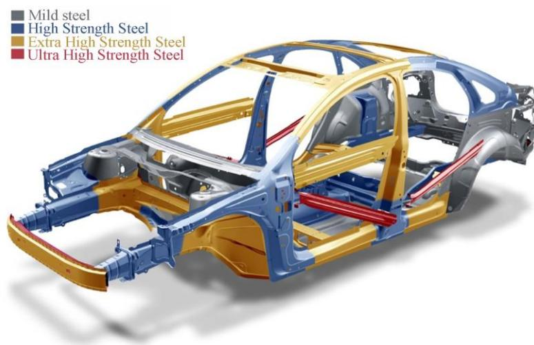
Figure 3 Steel types used in car body [16].
