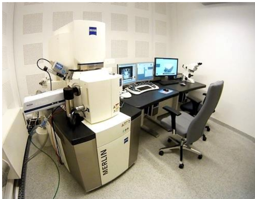
Figure 67. SEM Merlin Gemini II (ZEISS) [90]
