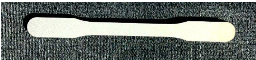
Figure 58. Conventional flat test specimen – real after production process.
