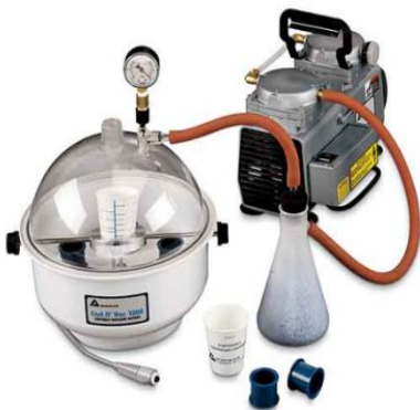
Figure 71. Vacuum Inclusion system Cast N' Vac 1000 [92]
