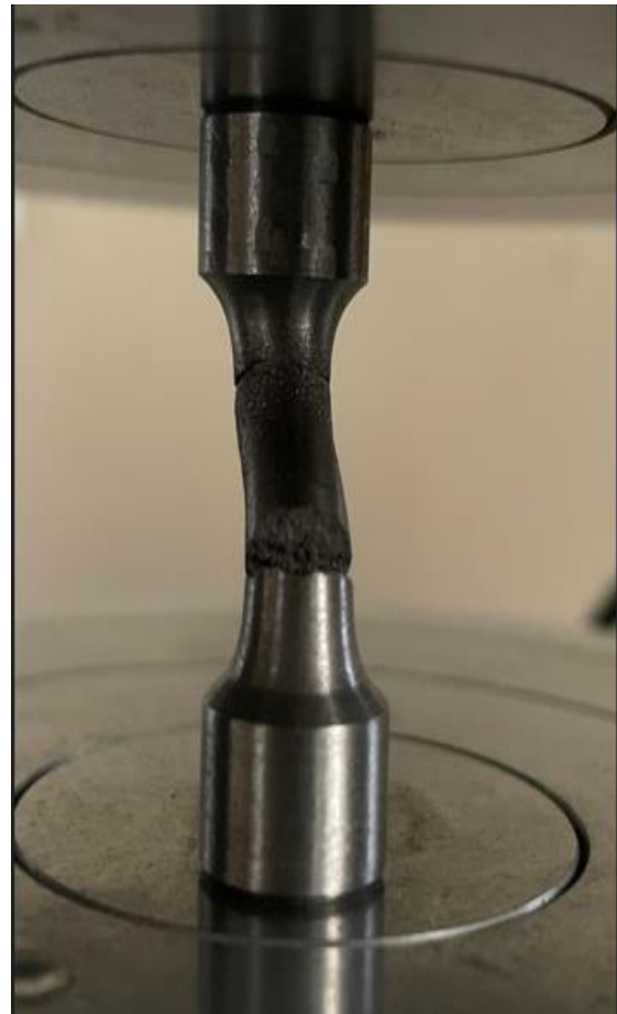
Figure 114. The sample after compression strength test.
