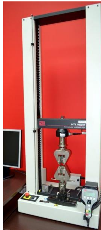
Figure 60. MTS Insight System 10kN [83]
