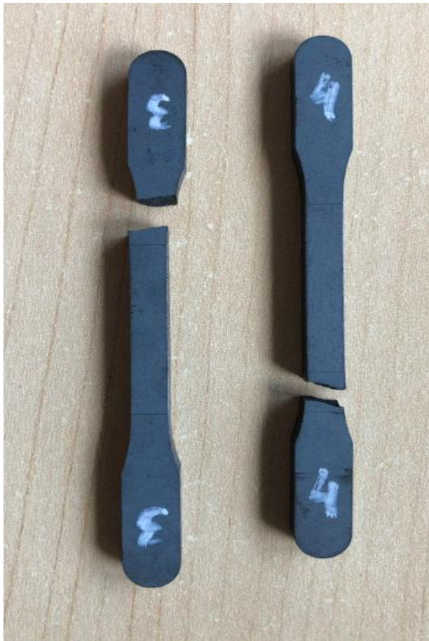
Figure 113. The sample after tensile strength test.
