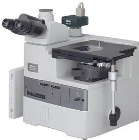
Figure 65. The optical microscope Eclipse MA200 NIKON [87]
