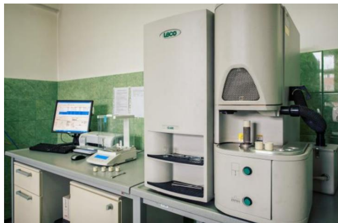
Figure 66. Carbon and sulphur content analyser - CS600 by LECO. [88]
