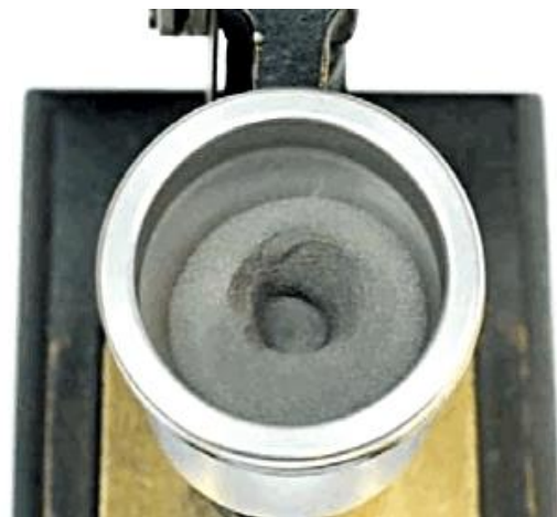
Figure 2. Flow patterns in Gustavsson Flowmeter [8].
