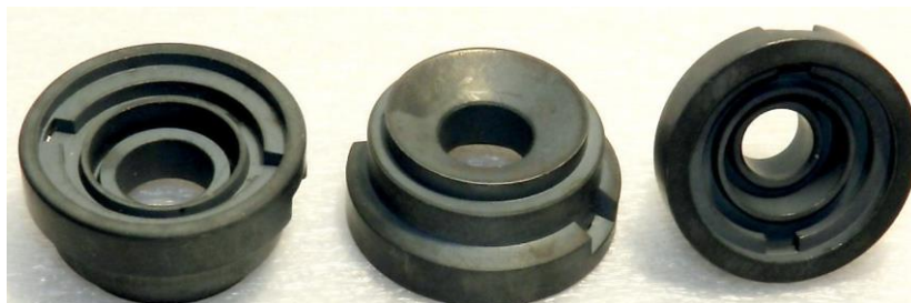
Figure 35. Powder Materials parts used in shock absorbers. [66]
