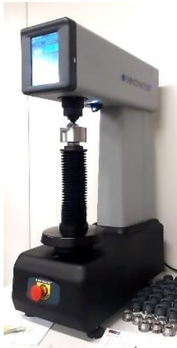
Figure 64. Rockwell hardness tester, manufacturer INNOVATEST, model VERZUS 710RS [86]
