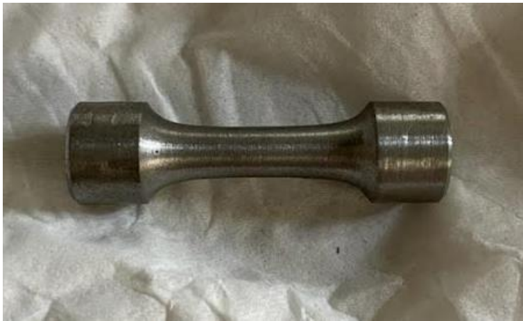
Figure 62. The produced compact for compression strength test according to norm [51]
