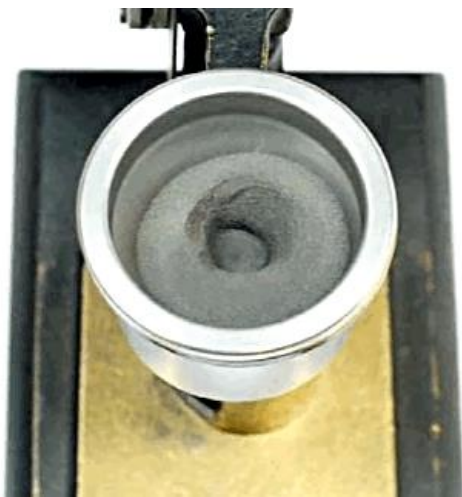
Figure 1. Flow patterns in Hall Flowmeter [8]
