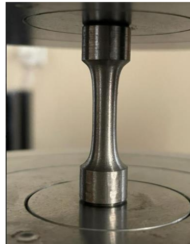
Figure 62. The produced compact for compression strength test according to norm [51]
