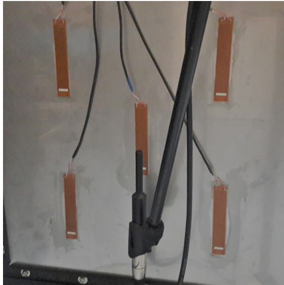
Figure 8: MFC elements glued to the radiating panel of the casing's double wall.
