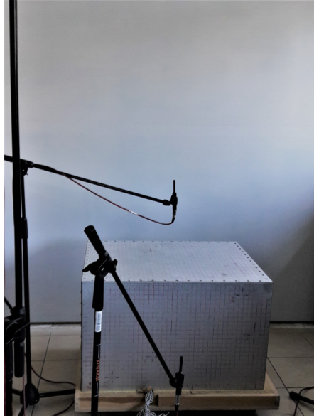
Figure 11: Experimental setup of the lightweight device casing placed at a wall.
