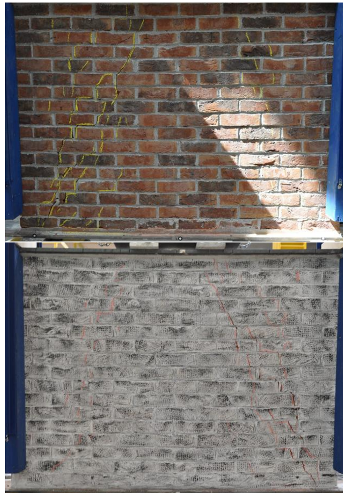
Figure 84: Crack patterns on back and front views of the wall made of mortar VS_129_350.
