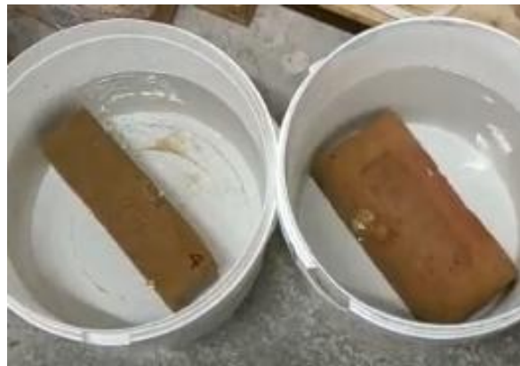
Figure 36: Full size units in submersion for water absorption measurements.
