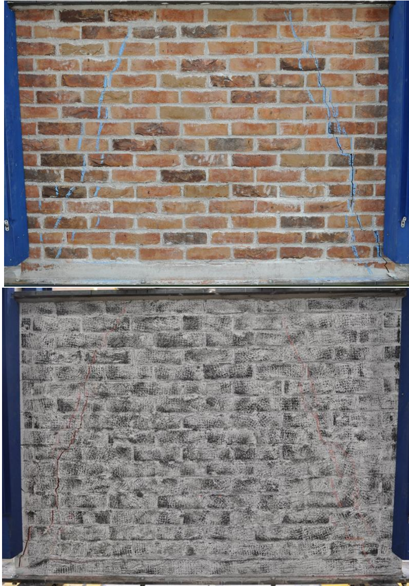
Figure 89: Crack patterns on back and front views of the wall made of mortar VS_129_600.
