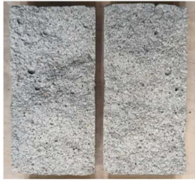
Figure 51: Typical failed sample after splitting load for both mortars. Adapted from Zagaroli et al. [212].
