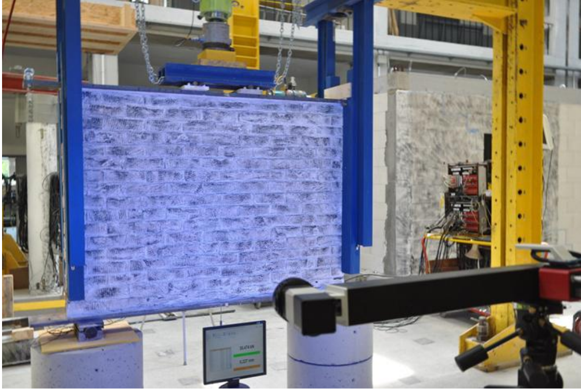
Figure 70: Test set-up for in-plane vertical shearing quasi-static test adopted in this study.
