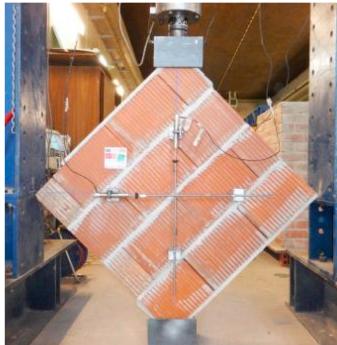
Figure 17: Typical test set up scheme for diagonal compressive test on masonry wallettes. From Silva et al. [106].
