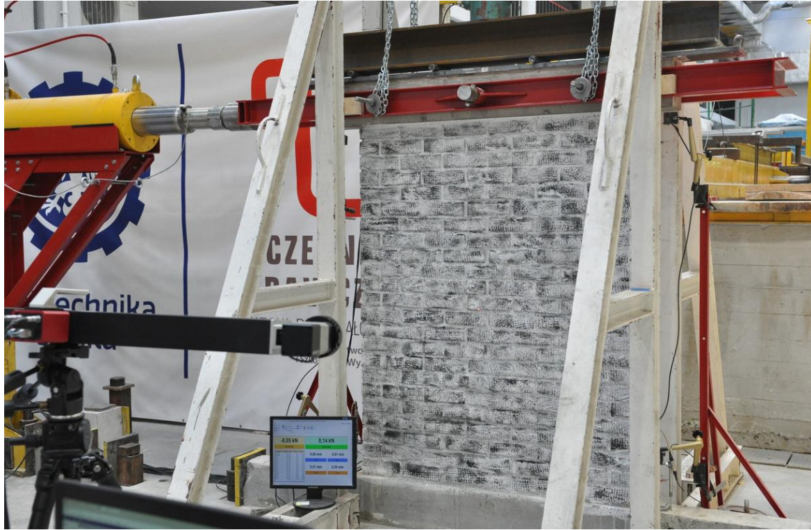
Figure 95: Test set-up for the lateral cyclic response with wall ready to be tested.
