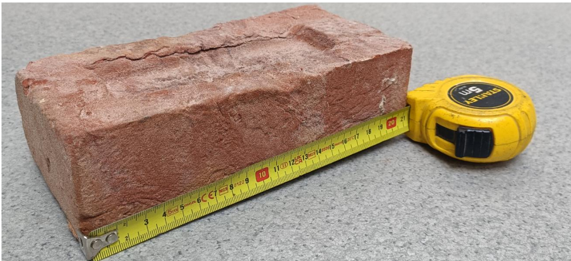
Figure 35: View of the frogged clay solid bricks used in presented investigations.
