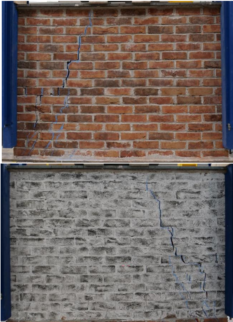
Figure 74: Crack patterns on back and front views of the wall made of mortar VS_116_350.
