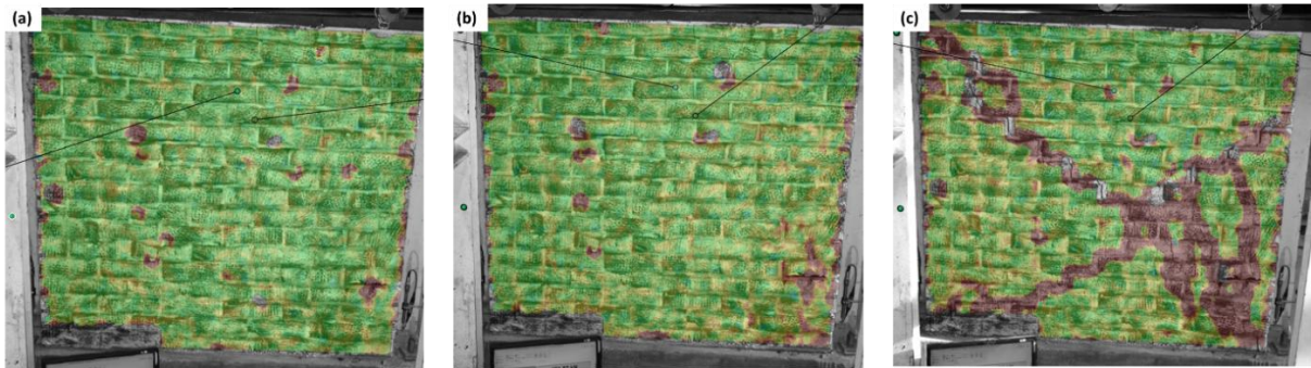
Figure 107: Initial shear response with limited damage (a), reduction in base shear due to rocking and concentration of cracks at the corner (b), and (c) crack pattern in correspondence of the failure for masonry wall HC_116_B_15.
