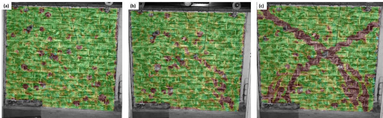
Figure 109: First visible crack formation (a), propagation of previous cracking (b), and (c) final diagonal cracking for masonry wall HC_129_B_15.
