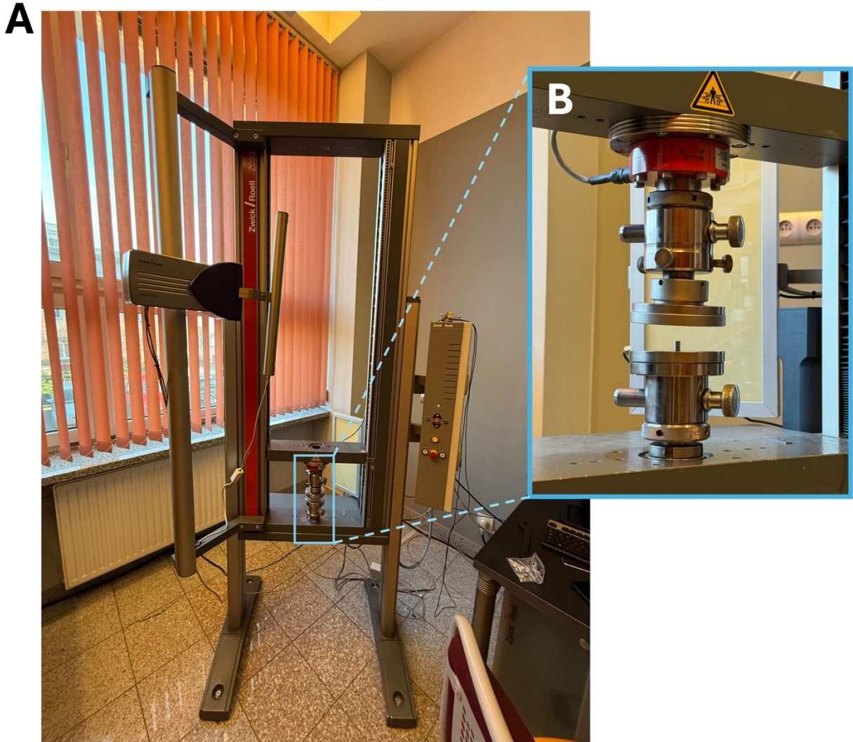
Figure 15. Zwick/Roell Z020 universal testing machine used for compression testing. A. View of the machine in the laboratory, and B. A closeup view of the crosshead of the compression testing system with a sample mounted on the lower head.
