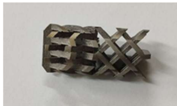
Figure 4. Photographs of the single ( left ) and double ( right ) static mixers.
