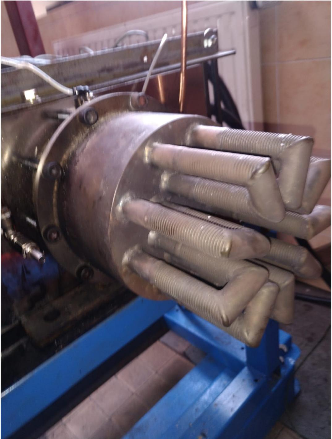
Figure 3.10: Outside view of the heater tubes
