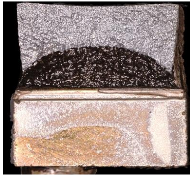
Creep degraded straight notch (C1)
