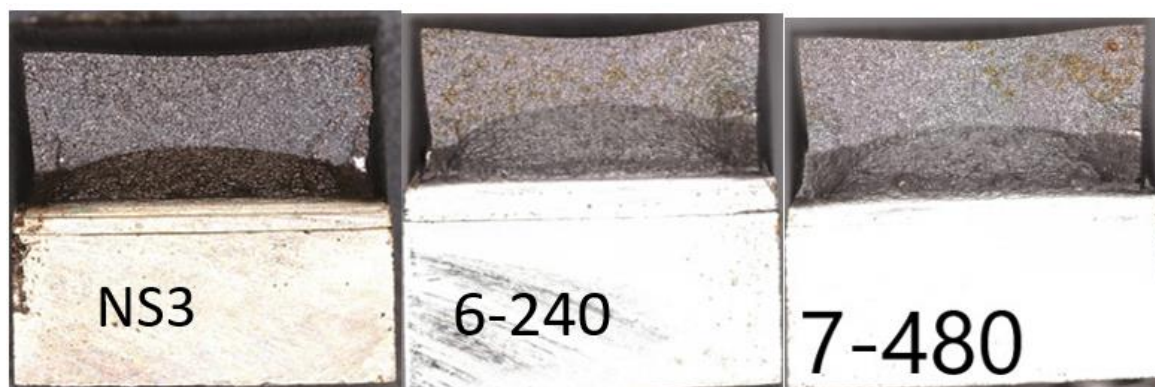
FIGURE 70: Fracture surface showing the crack front of new and aged specimen.
