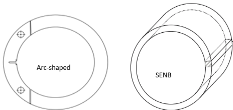
FIGURE 35: A schematic diagram showing the sampling position of the arc tension and SENB specimens.
