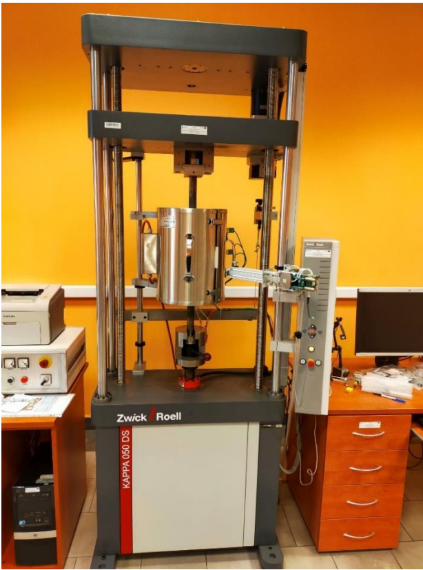
FIGURE 71: The 50 kN capacity kappa 050 ds Zwick/Roell creep testing machine fitted with controlled furnaces.
