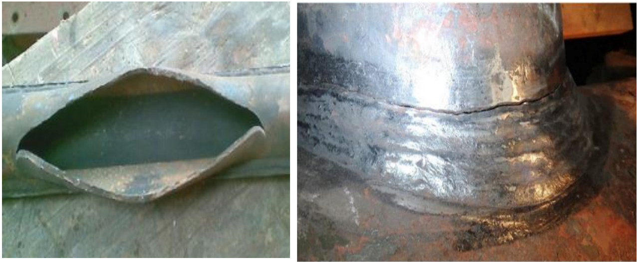
FIGURE 1: Ruptured boiler tube (a) [5], damage to the welding that connected the collector to the communication tubes (b) [12].
