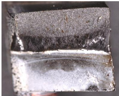
Creep degraded straight notch (C1)
