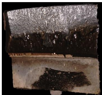
Creep aged 45-degree notch (4C)
