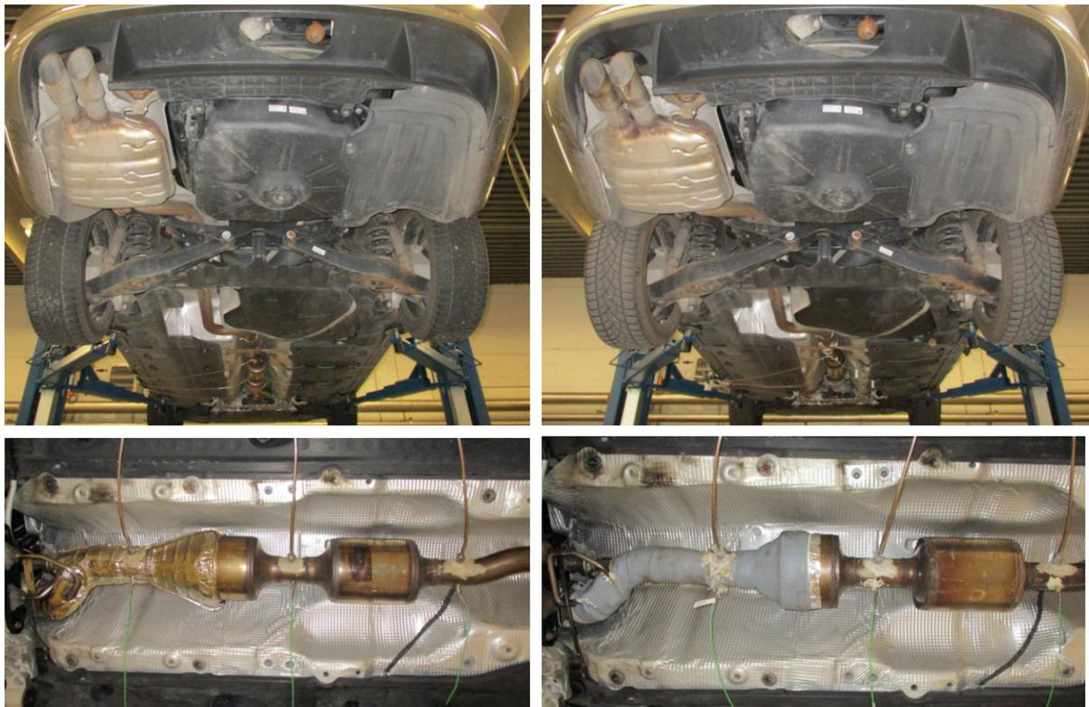
Fig. 120. Installed OEM and WALKER SCR systems under the car with sampling points
