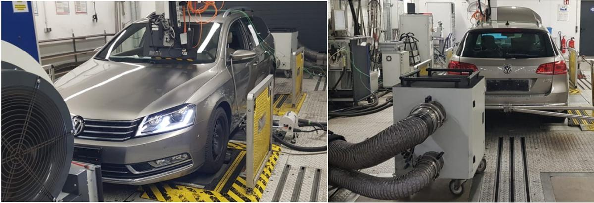
Fig. 121. Car prepared for emission tests on chassis dynamometer
