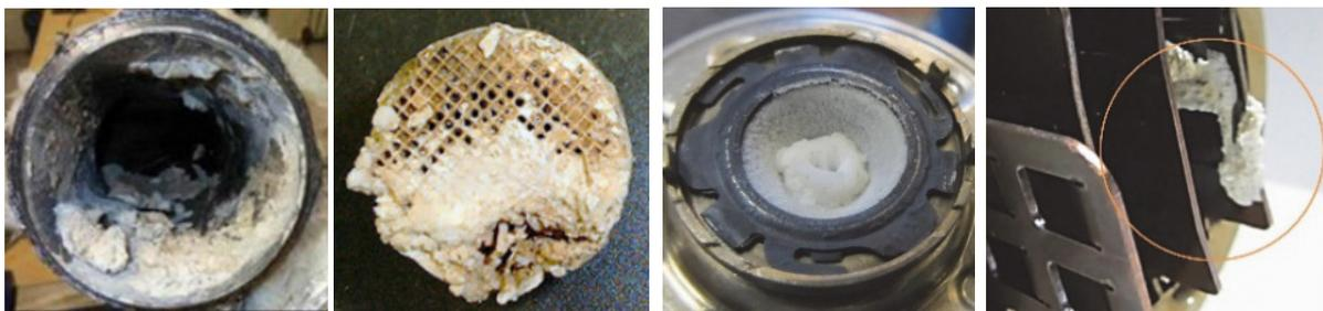
Fig. 46. Deposit formation on the pipe, catalyst, injector and mixer [116], [120]
