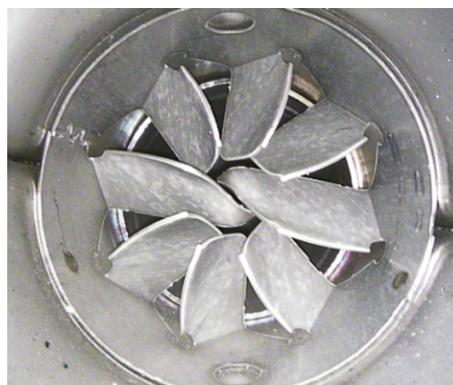
Fig. 56. Endoscopic photo of the original mixer
