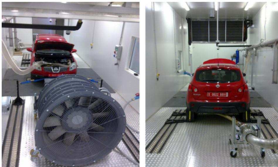
Fig. 27. Front (left) and back (right) of the roller test bench under climatic chamber [66]
