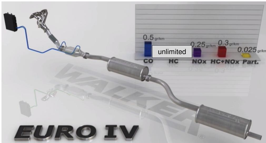
Fig. 21. Example of an exhaust system for Euro 4 (Category M<sub>1</sub>, Diesel) [60]
