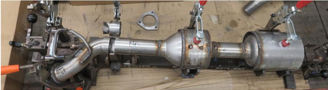
Fig. 52. Fixture in the phase of construction of a prototype of the SCR
