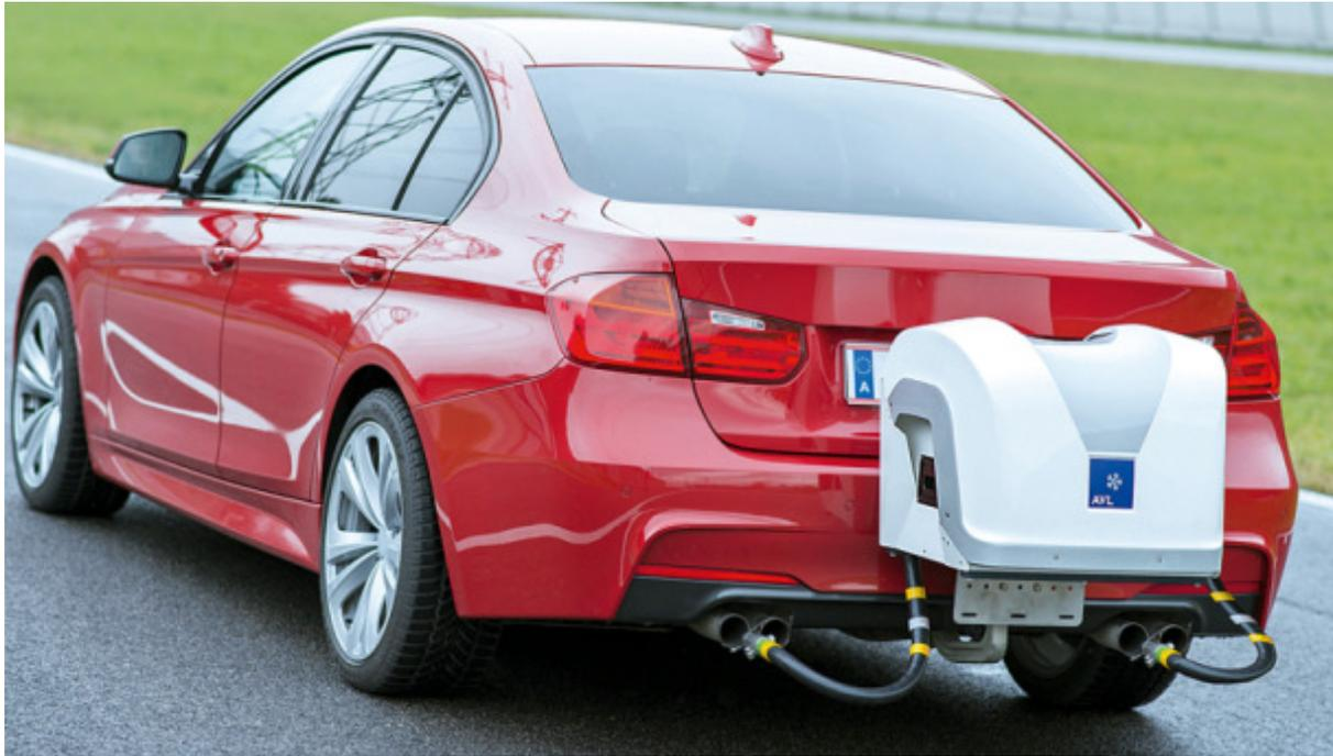
Fig. 29. Portable Measurement Systems (PEMS) on a vehicle [70]
