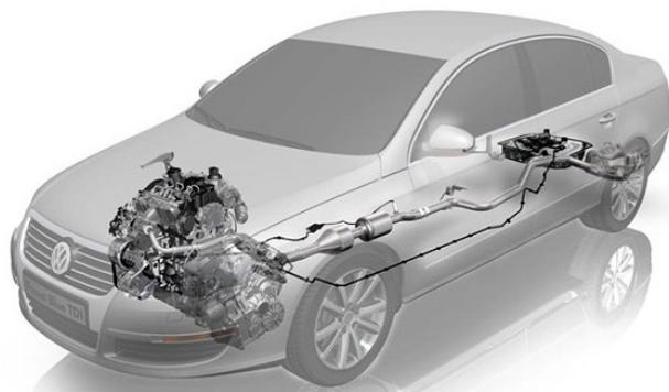
Fig. 49. Car with the tested SCR system [130]
