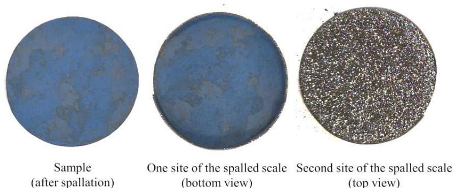
Figure 5.6: Macrographs showing the ORE sample after severe oxide spallation during long-term cyclic oxidation at 900 °C.
