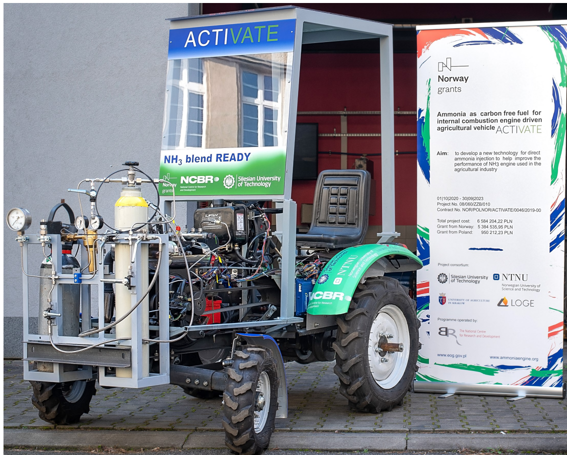
FIGURE 6.1: Liquid ammonia-biodiesel fueled prototype agriculture tractor
