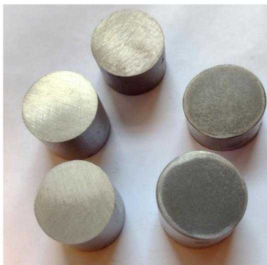
Figure 18. Specimens EN AC-Al Si12CuNiMg of the alloy for the hardness test
