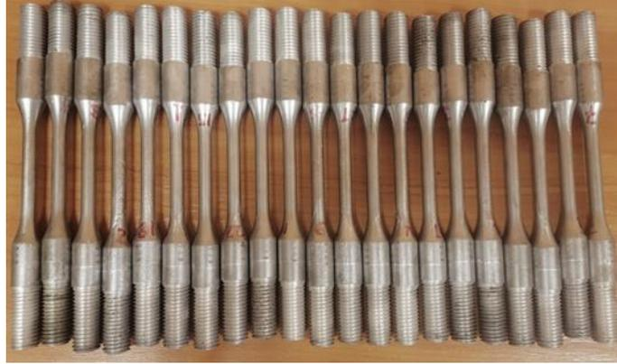
Figure 30. Tensile specimens of composite material
