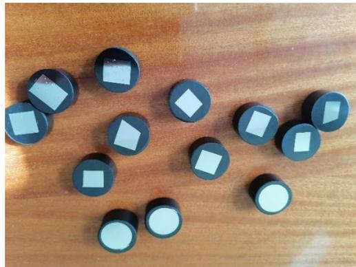
Figure 26. Metallographic specimens
