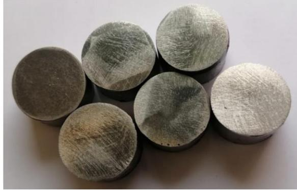
Figure 38. Hardness test specimens of the composite material
