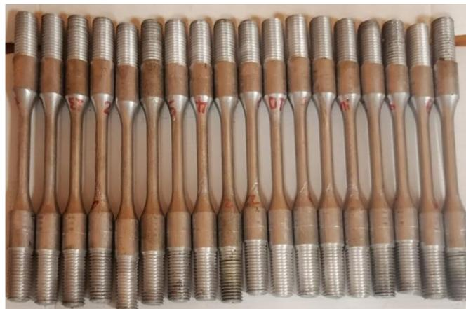
Figure 43. The prepared fatigue, relaxation, and creep test specimens
