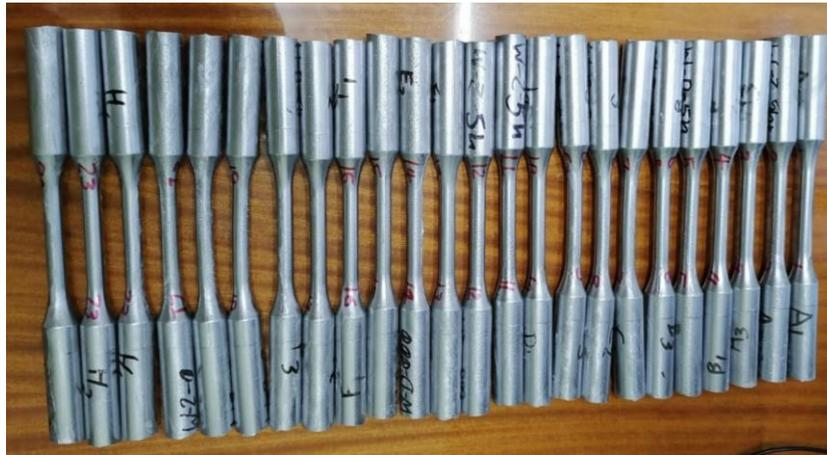
Figure 10. Tensile specimens
