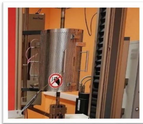
Figure 44. Fatigue, relaxation, and creep test set-up
