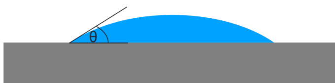
Figure 3 Schematic diagram of the contact angle ( \theta ).
