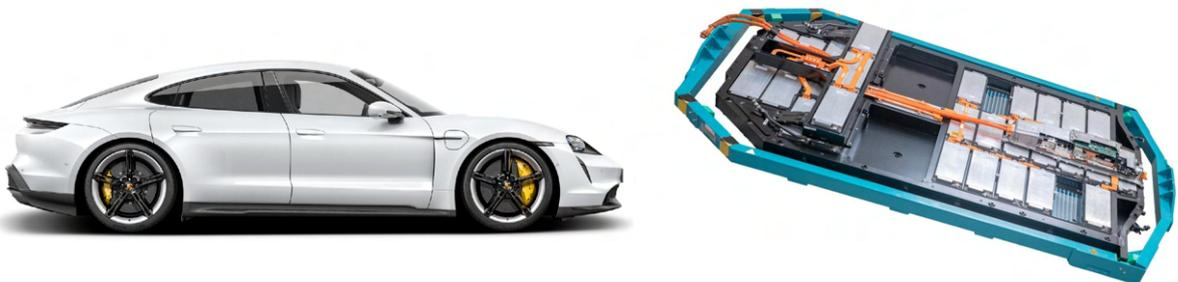
**Fig. 1.4.** Porsche Taycan and 3D model of its battery pack [10]
