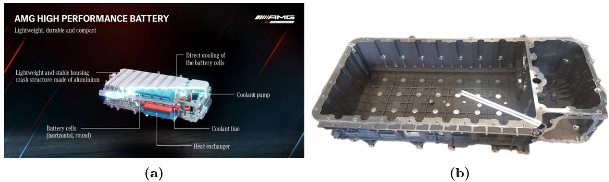
**Fig. 4.4.** (a) HPB80 battery pack with immersive cooling [133] (b) Bottom part of the HPB80's battery pack housing
