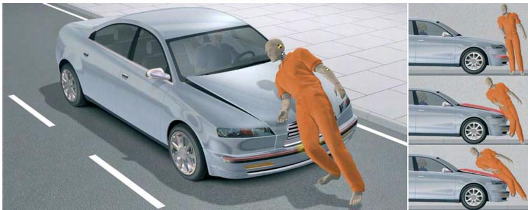
**Fig. 3.10.** Pedestrian protection system [127]
