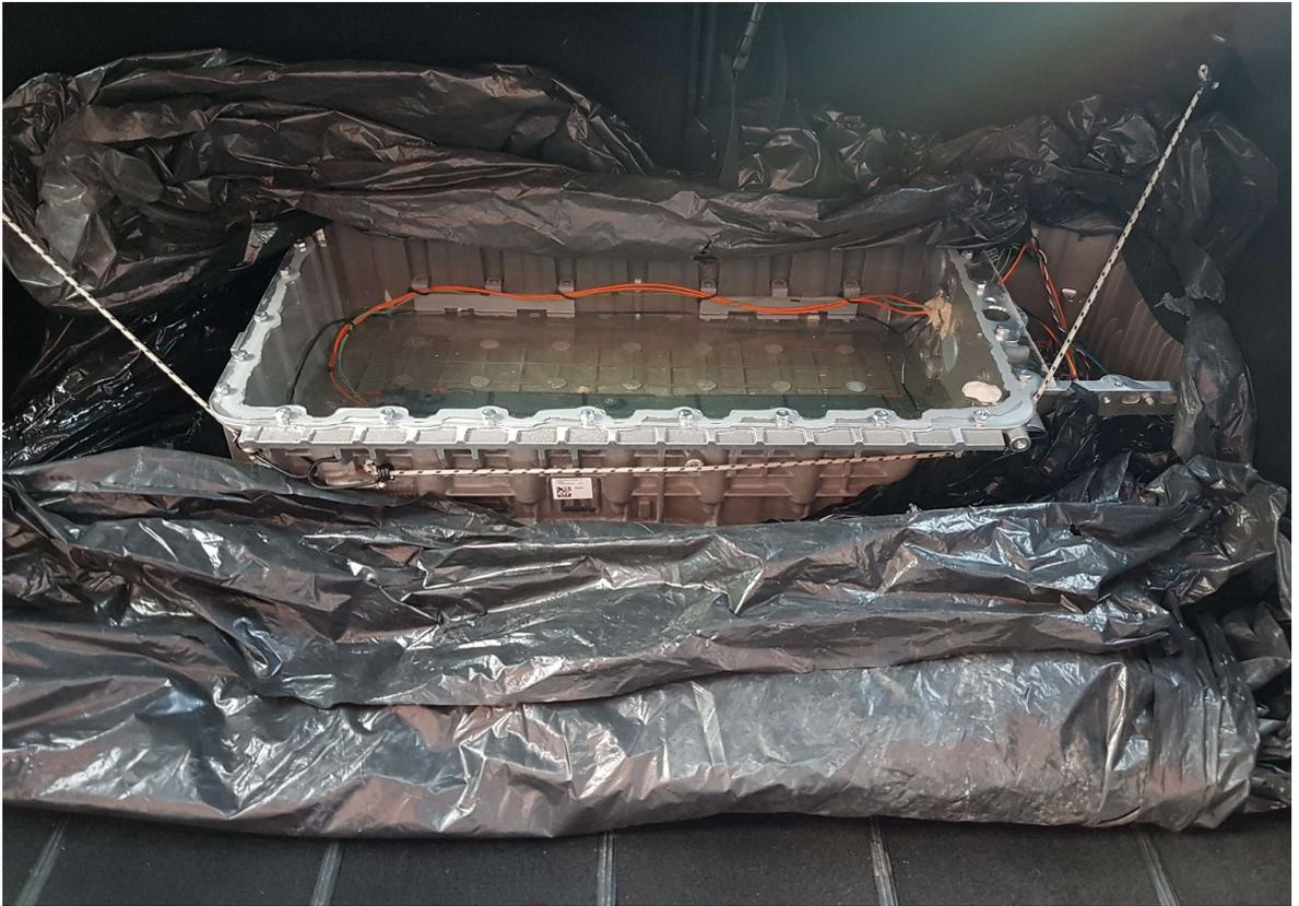
**Fig. 6.14.** Optical liquid detection system installed inside the vehicle
