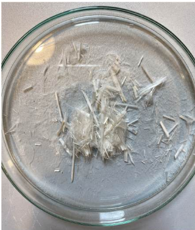
Fig. 3. Recovered glass fibers after the process.
