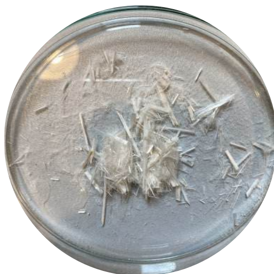
Figure 3.1 Pure glass fibres obtained from oxidative liquefaction of WTBs
