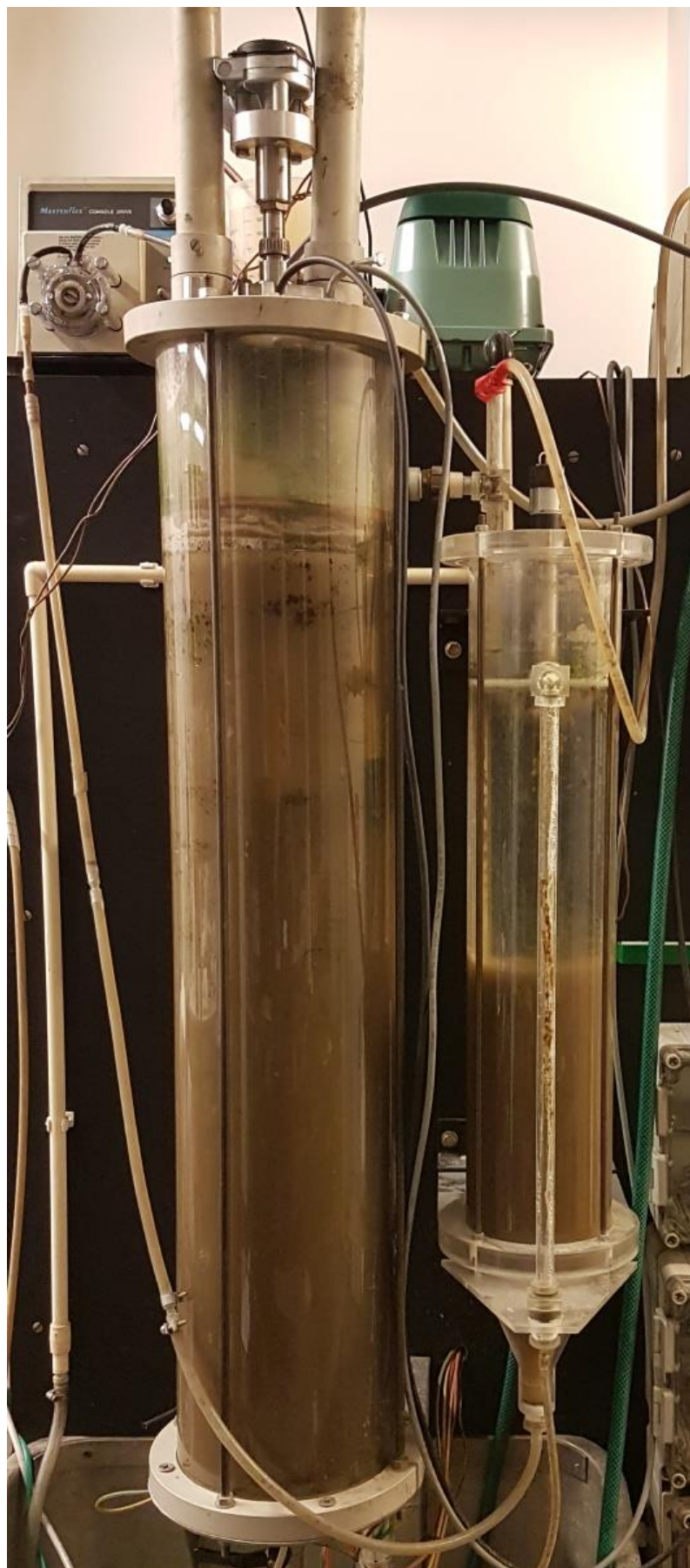
Fig. 3.2 Laboratory scale wastewater treatment test plant used in MAS verification
