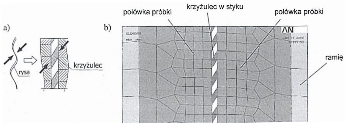
Fig. 3.63. Modelling the interface through diagonal cross-bracing: a) idea, b) finite element system [59]
