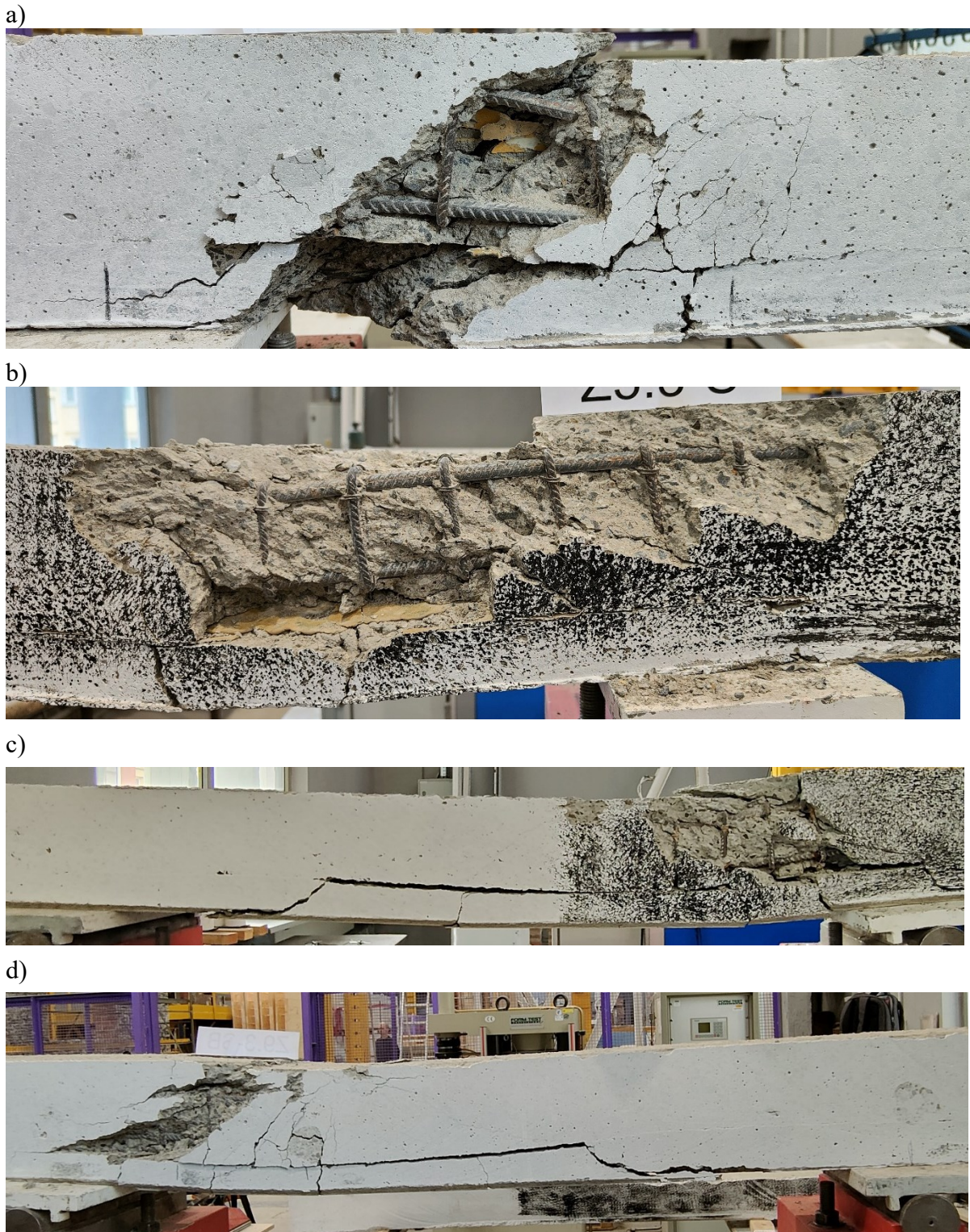
Fig. 6.53. View beams after failure: a) Z4.3_P, b) Z5.3_S, c) Z9.3_SB, d) Z10.3_TS
