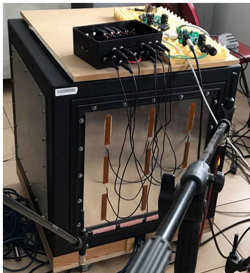
Figure 3.7: Rigid device casing with MFC elements used in experiment [53].
