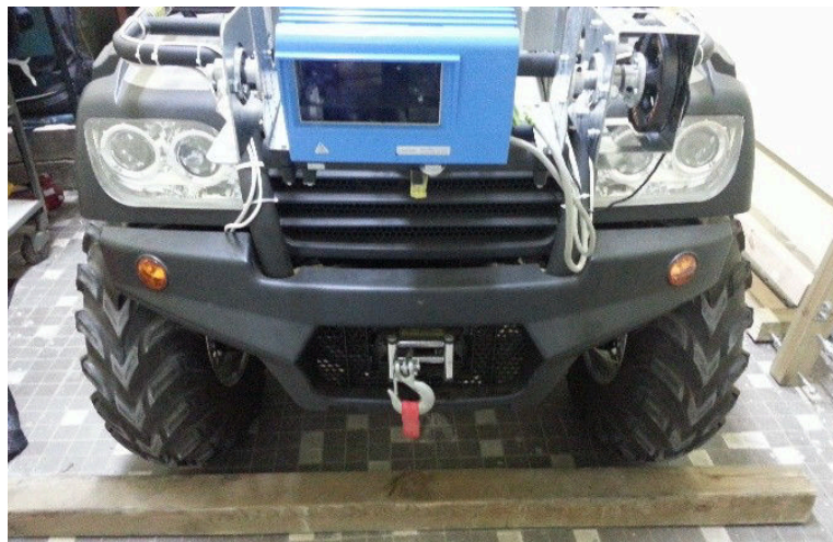
Figure 5.4: 0.08 m thick wooden beam, used as an obstacle, compared with investigated vehicle.
