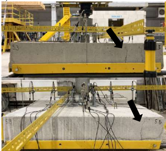
Fig. 5.47 Location of first (grey arrow), second (black arrow), and further (white arrow) flexural cracks of tested slabs of type 5 (PD_3)
