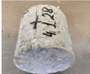
Fig. 5.3 Selected drilled cores after the splitting tensile tests
