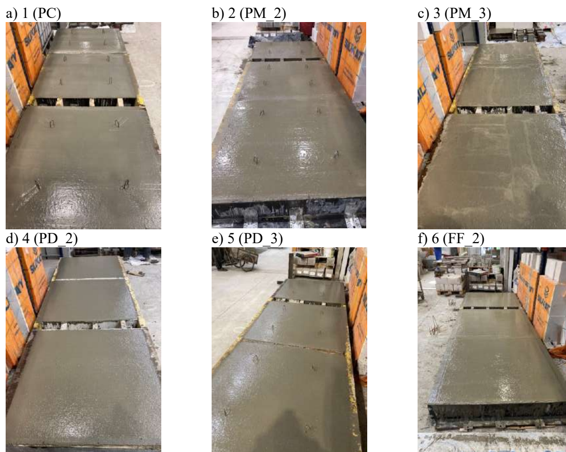
Fig. 4.4 Large-scale slab samples after concreting
