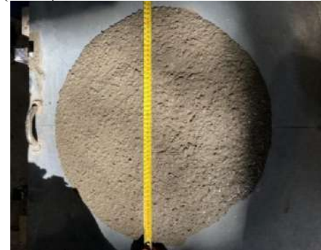
Fig. 5.1 View of slumps of tested concrete mixture during the flow table tests
