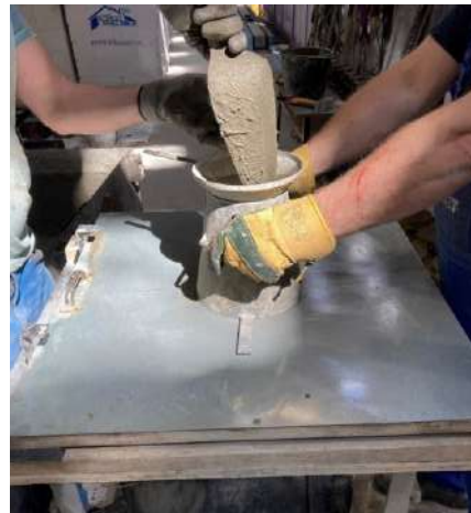
Fig. 4.6 Flow table test: a) testing apparatus [208], b) filling the cone during the test
