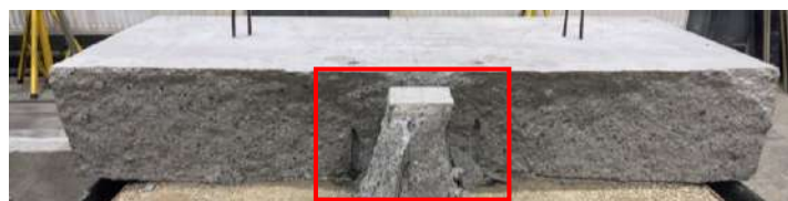
Fig. 5.52 Fractured side surface of the ground slabs type 1 (PC)
