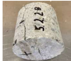
Fig. 5.3 Selected drilled cores after the splitting tensile tests
