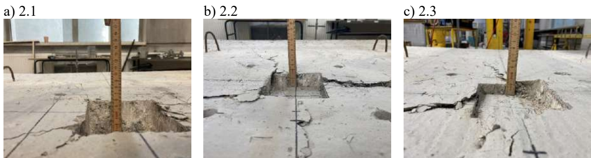
Fig. 5.29 Punching of the tested slabs of type 2 (PM_2) at the load application surface
