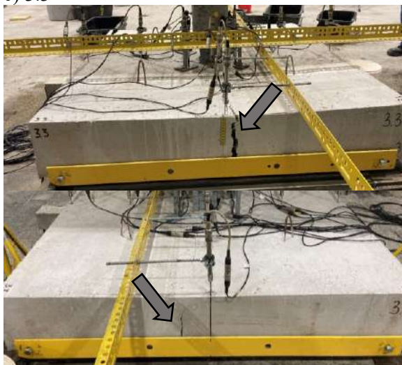
Fig. 5.33 Location of first (grey arrow), second (black arrow), and third (red arrow) flexural cracks of tested slabs of type 3 (PM_3)
