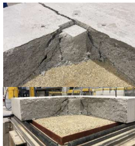
Fig. 5.20 Crack pattern of tested slabs of type 1 (PC): first (grey curve), and second (black curve) flexural cracks
