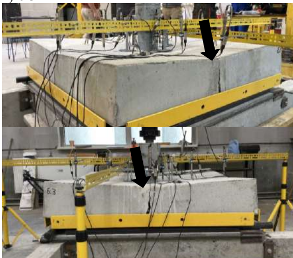
Fig. 5.12 Location of first (grey arrow), second (black arrow), and further (white arrow) flexural cracks of tested slabs of type 6 (FF_2)
