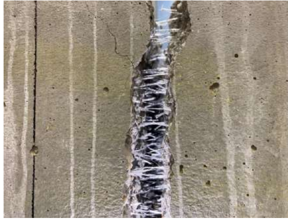
Fig. 5.39 Synthetic fibers PD maintaining the structural integrity of the tested slab 4.2
