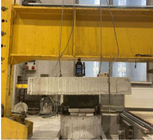
Fig. 4.26 Setup for punching shear cone removal from the tested slabs
