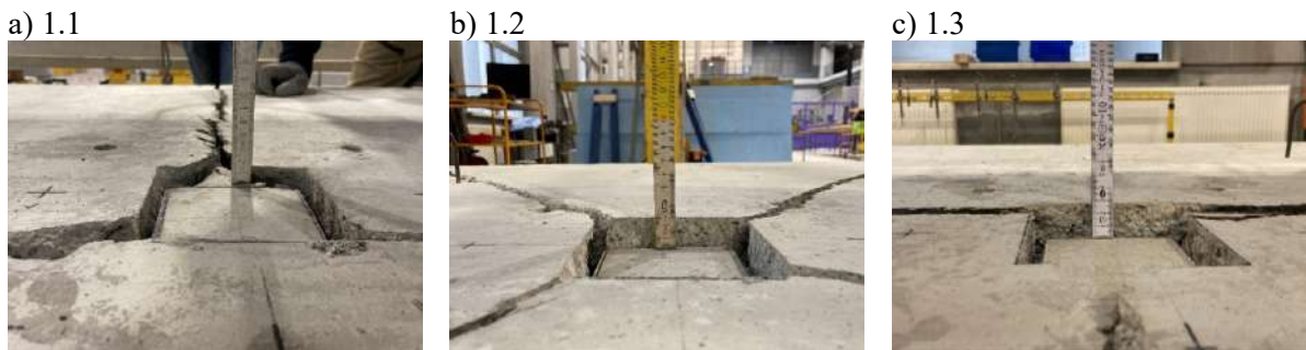
Fig. 5.22 Punching of the tested slabs of type 1 (PC) at the load application surface
