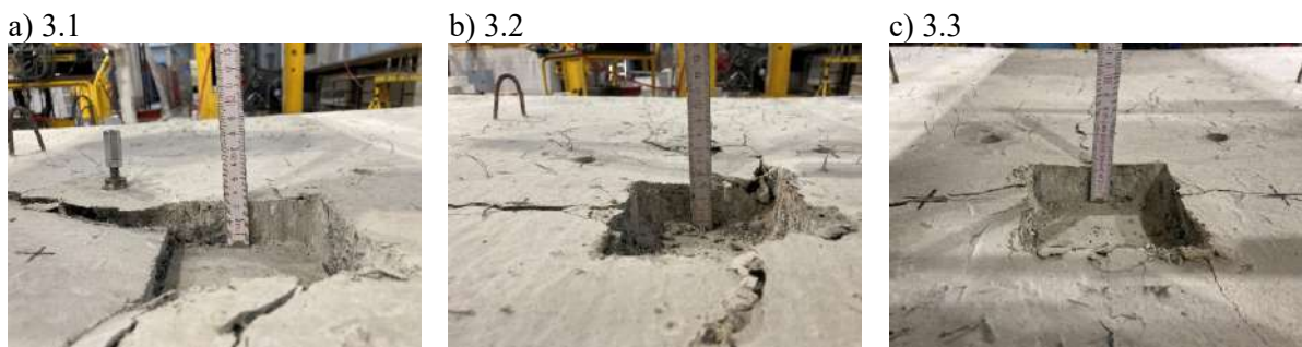
Fig. 5.36 Punching of the tested slabs of type 3 (PM_3) at the load application surface
