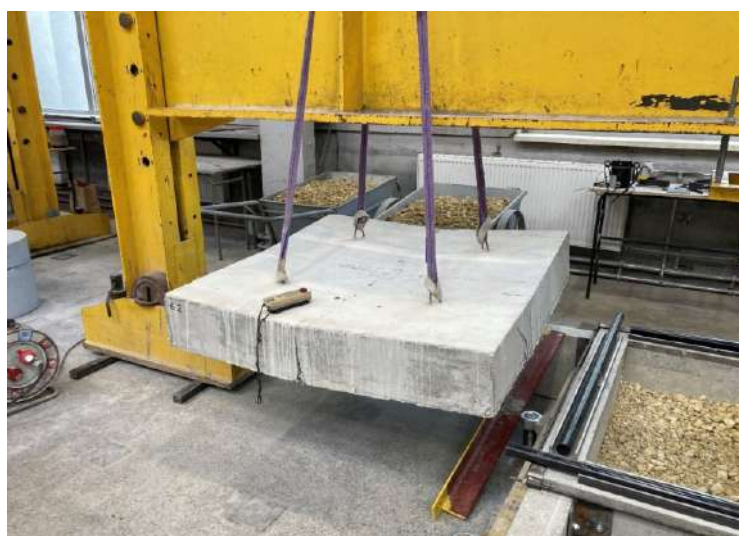
Fig. 4.16 Slab 6.2 after the test exclusively on four steel supporting rollers, without ground support
