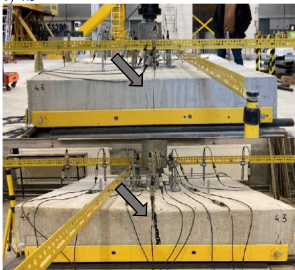
Fig. 5.40 Location of first (grey arrow), and second (black arrow) flexural cracks of tested slabs of type 4 (PD_2)
