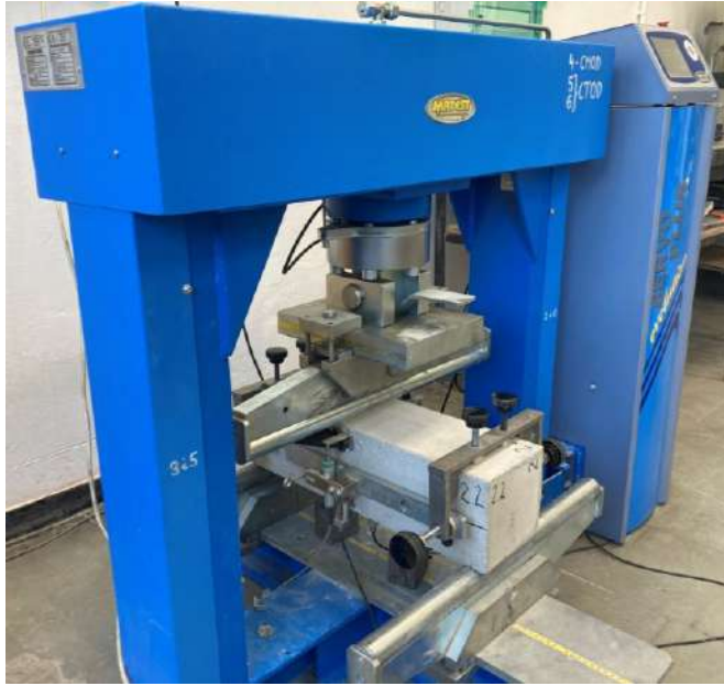
Fig. 4.12 View of the setup during the 3PBT with the location of measurement devices, where: 5 – LVDT to measure \delta ; 6 – clip gauge to measure CTOD ; 7 – clip gauge to measure CMOD
