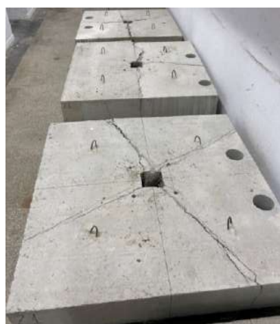
Fig. 4.5 Tested slabs of type 2 with holes remaining from core drilling
