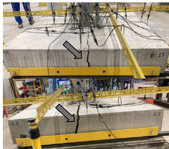
Fig. 5.19 Location of first (grey arrow), and second (black arrow) flexural cracks of tested slabs of type 1 (PC)
