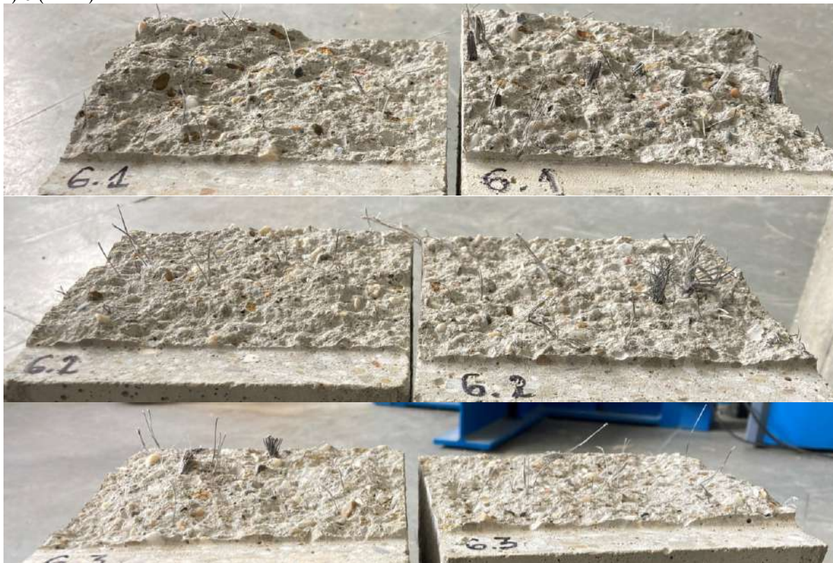
Fig. 5.7 Notch cross-section of broken beams after 3PBT (fiber distribution)
