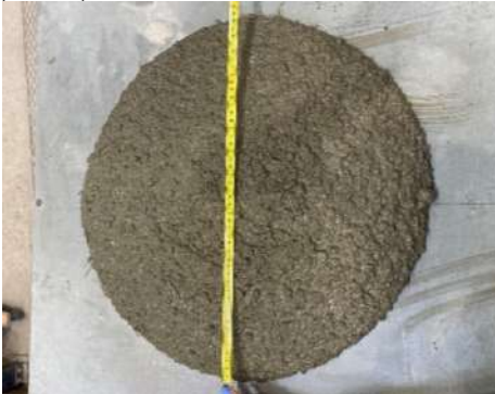
Fig. 5.1 View of slumps of tested concrete mixture during the flow table tests
