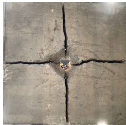
Fig. 5.17 Bottom surface of the ground slabs type 6 (FF_2) after removal of the punching cone
