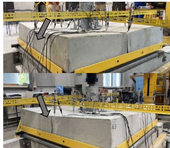
Fig. 5.12 Location of first (grey arrow), second (black arrow), and further (white arrow) flexural cracks of tested slabs of type 6 (FF_2)
