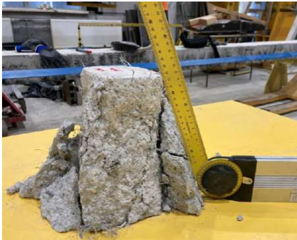
Fig. 4.27 Measurement of punching shear cone inclination angles \theta using an angle finder ruler
