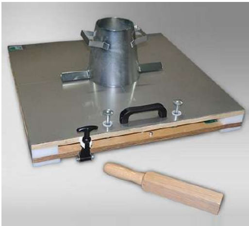
Fig. 4.6 Flow table test: a) testing apparatus [208], b) filling the cone during the test
