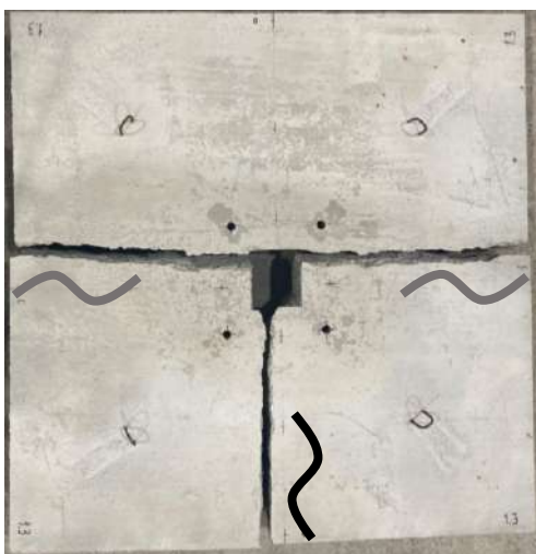
Fig. 5.20 Crack pattern of tested slabs of type 1 (PC): first (grey curve), and second (black curve) flexural cracks
