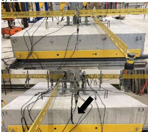
Fig. 5.19 Location of first (grey arrow), and second (black arrow) flexural cracks of tested slabs of type 1 (PC)
