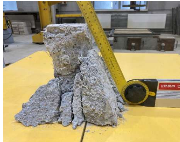
Fig. 4.27 Measurement of punching shear cone inclination angles \theta using an angle finder ruler
