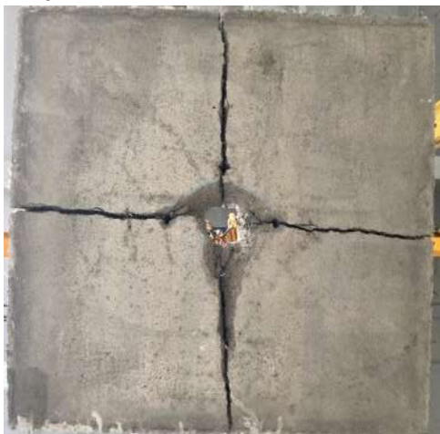
Fig. 5.17 Bottom surface of the ground slabs type 6 (FF_2) after removal of the punching cone
