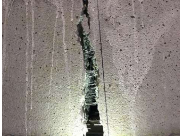
Fig. 5.11 Synthetic fibers FF maintaining the structural integrity of the tested slab 6.3
