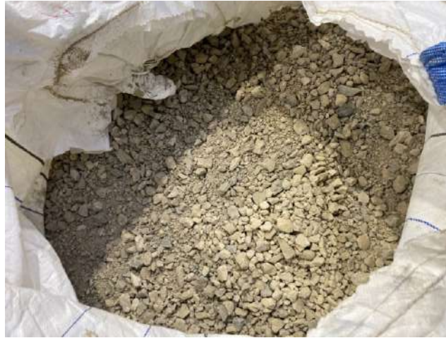
Fig. 4.2 Aggregates used to support the ground slabs in large-scale tests
