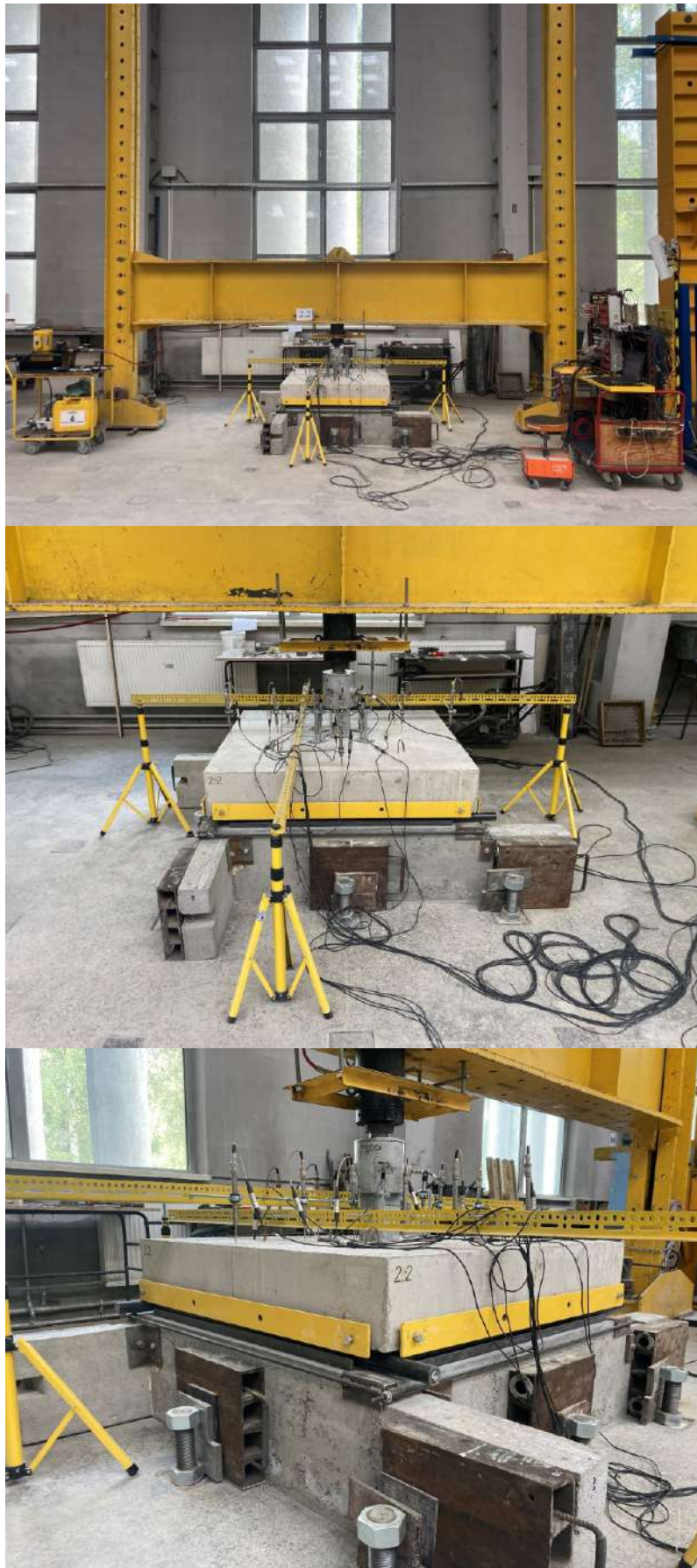
Fig. 4.21 Testing setup for ground-supported slabs centrally loaded by a concentrated force
