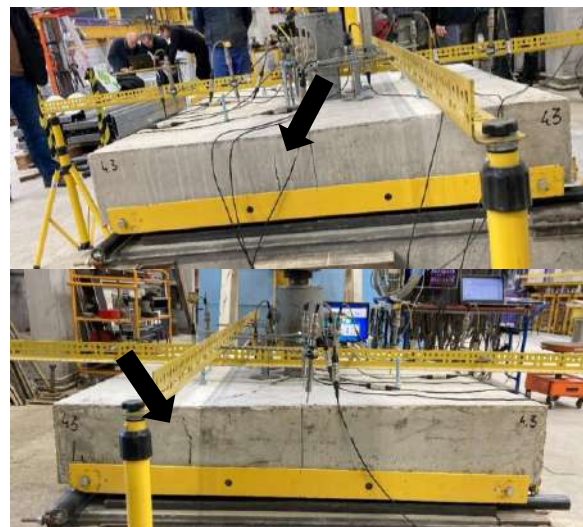
Fig. 5.40 Location of first (grey arrow), and second (black arrow) flexural cracks of tested slabs of type 4 (PD_2)
