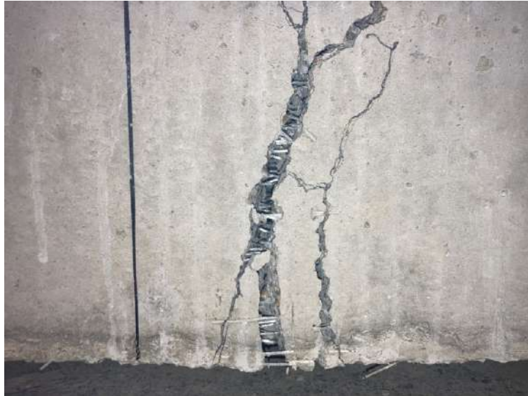
Fig. 5.46 Synthetic fibers PD maintaining the structural integrity of the tested slab 5.3
