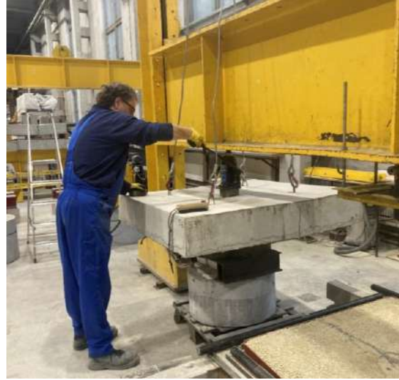
Fig. 4.26 Setup for punching shear cone removal from the tested slabs
