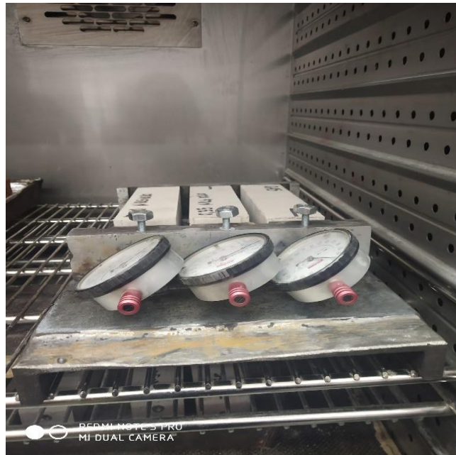
Figure 7. Measuring of dry shrinkage by Graf Kaufman Apparatus
