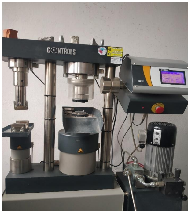
Figure 6. Universal machine for testing of Flexural and Compressive strength
