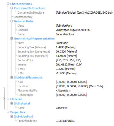
Fig. 3-3. Modeling IFC: superstructure's geometry and characteristics
