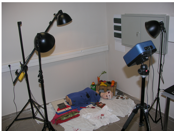
Figure 1.7: The picture of the local sensing stand with a hyperspectral camera and several halogen lamps.
