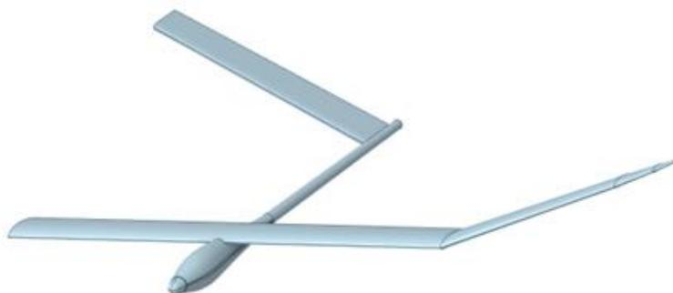
Figure 58 Simplify the model for aerodynamic analysis
