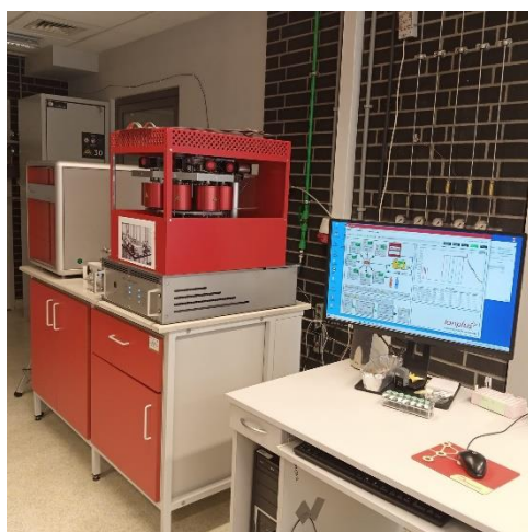
Fig. 1a Elemental Analyzer coupled with automated graphitization equipment at Gliwice 14 C and Mass Spectrometry Laboratory.
