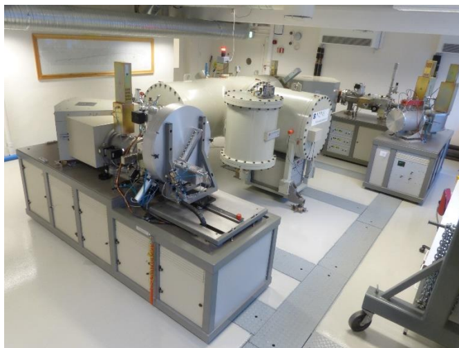
Fig. 2 Accelerator mass spectrometer at the National Laboratory for Age Determination, Trondheim, Norway.
