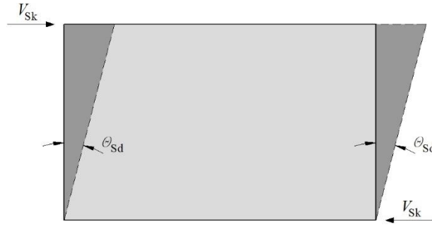
Fig. 3.6 Calculation model to determine the shear deformation angle \theta_{Sd} of a horizontally loaded stiffening wall
