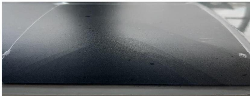
**Figure 8.8.** Damaged solar cell on the wing surface.
