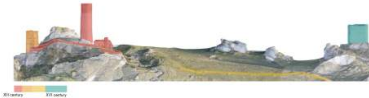
Fig. 205. The ability to date elements that are part of the complex elaborated by the author in Revit
