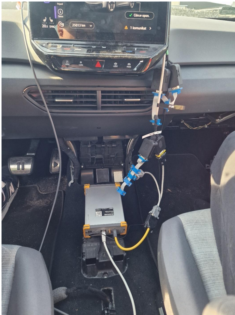
Fig. 58 Real car Microdaq E2000 device as a bridge connected to CAN bus
