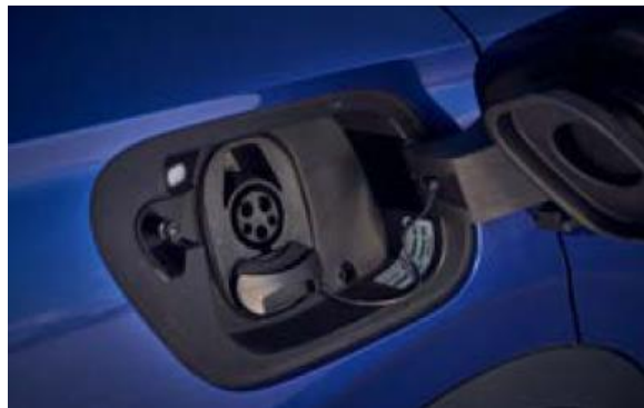
Fig. 21 High-Voltage Battery Charging Socket
