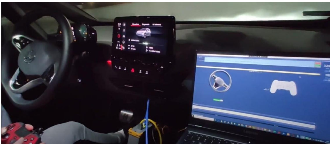
Fig. 78 Set of devices to take control of the steering gear system: MicroDAQ E2000 as a bridge, pad, notebook with PC application
