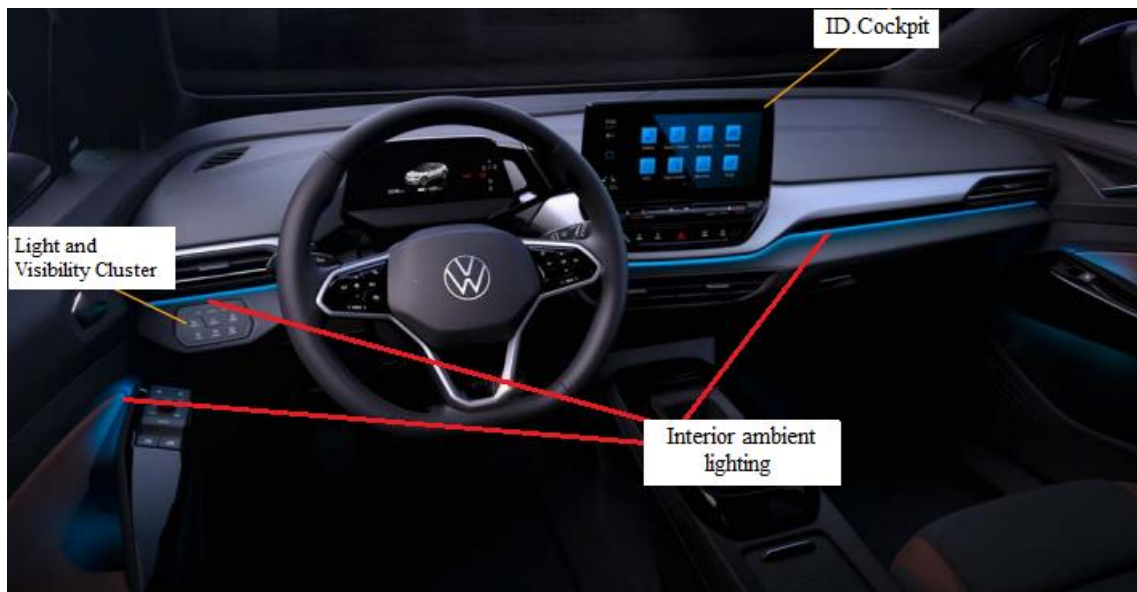
Fig. 38 Interior ambient lighting
