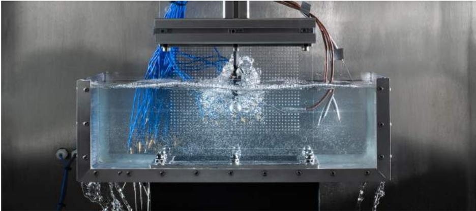
FIGURE 2.2: Flow of the refrigerating liquid over the artificial sample inside the HF tank at the test rig.
