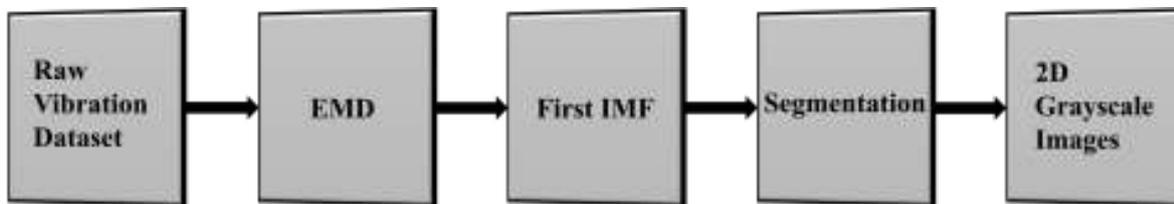
Figure 5.1: Block diagram for preprocessing steps.
