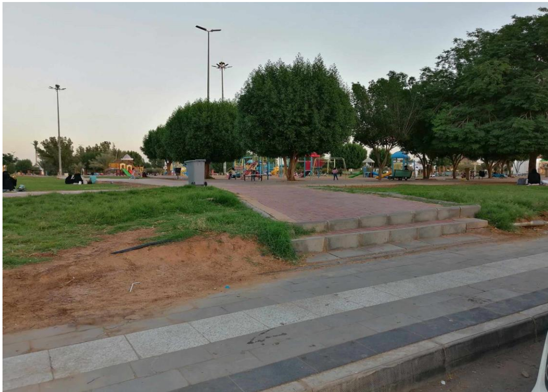
Figure 2. An example of a high curb and stairs along the main path of play space in King Fahd Central Park, Saudi Arabia.
