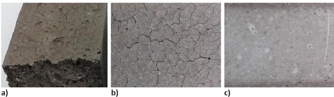
Fig.3.8.5: Samples cured at 20°C and demoulded after 24 hours (M/G 60/40): a) upper surface, b) side surface, c) bottom surface. Photos made after 7 days of curing.
