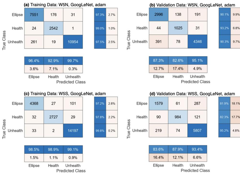
Figure 5.10: Orbit-shaped image CNN classification models of hanger dynamic behavior using one bi-directional vibration sensor: a) and b) for W5N; c) and d) for W5S.
