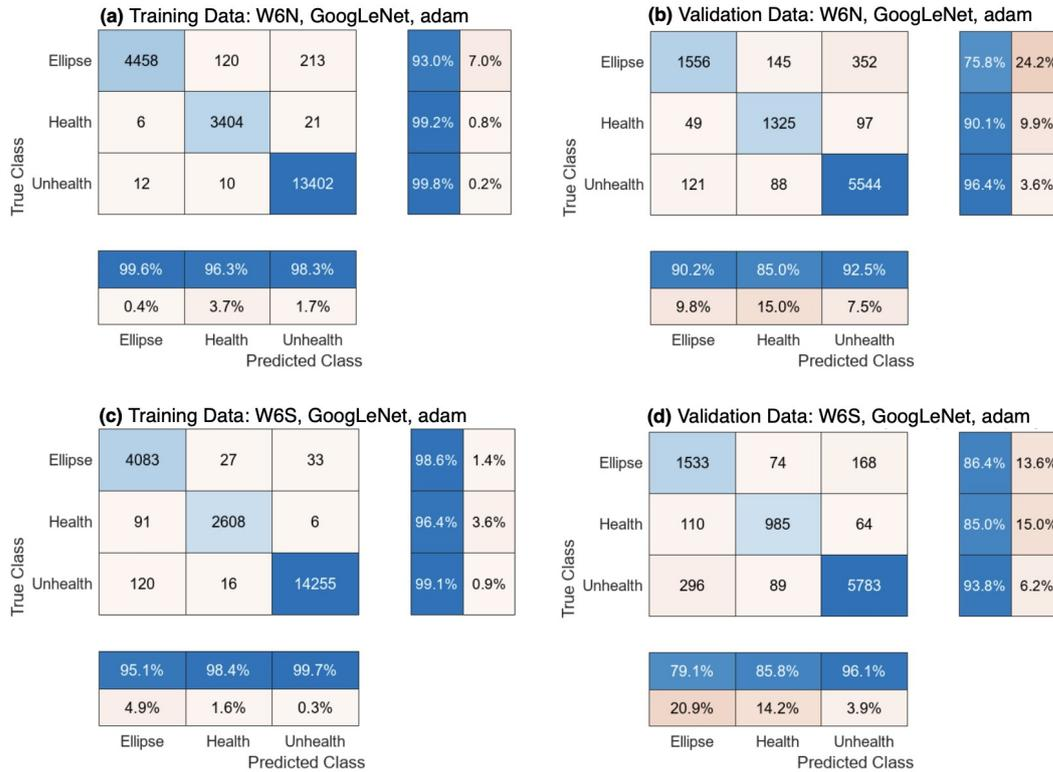
Figure 5.11: Orbit-shaped image CNN classification models of hanger dynamic behavior using one bi-directional vibration sensor: a) and b) for W6N; c) and d) for W6S.
