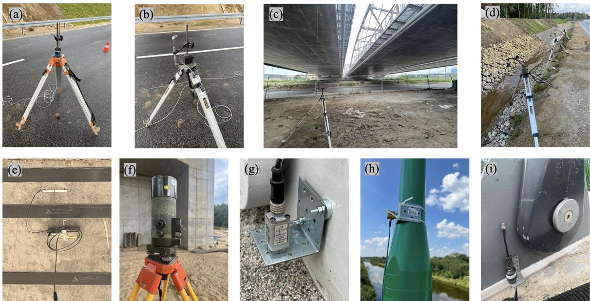
Figure 3.3: Instruments for bridge diagnostic testing in the field: a), b), c), d) deflection measurement; e) strain gauge sensor; f) Jenoptik Koni 007 for measuring span deflection and abutment displacement; g), h), i) vibration measurement.
