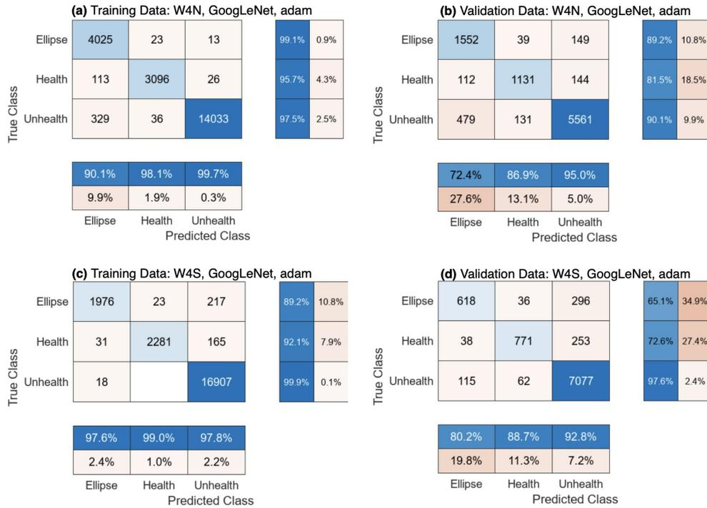
Figure 5.9: Orbit-shaped image CNN classification models of hanger dynamic behavior using one bi-directional vibration sensor: a) and b) for W4N; c) and d) for W4S.
