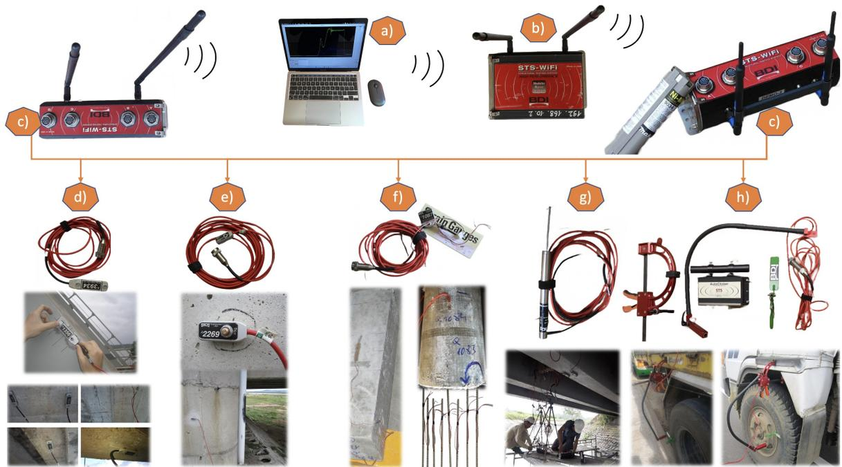
Figure 3.4: The wireless structural testing system (STS-WiFi) for diagnostic load testing of existing bridge structures [8].
