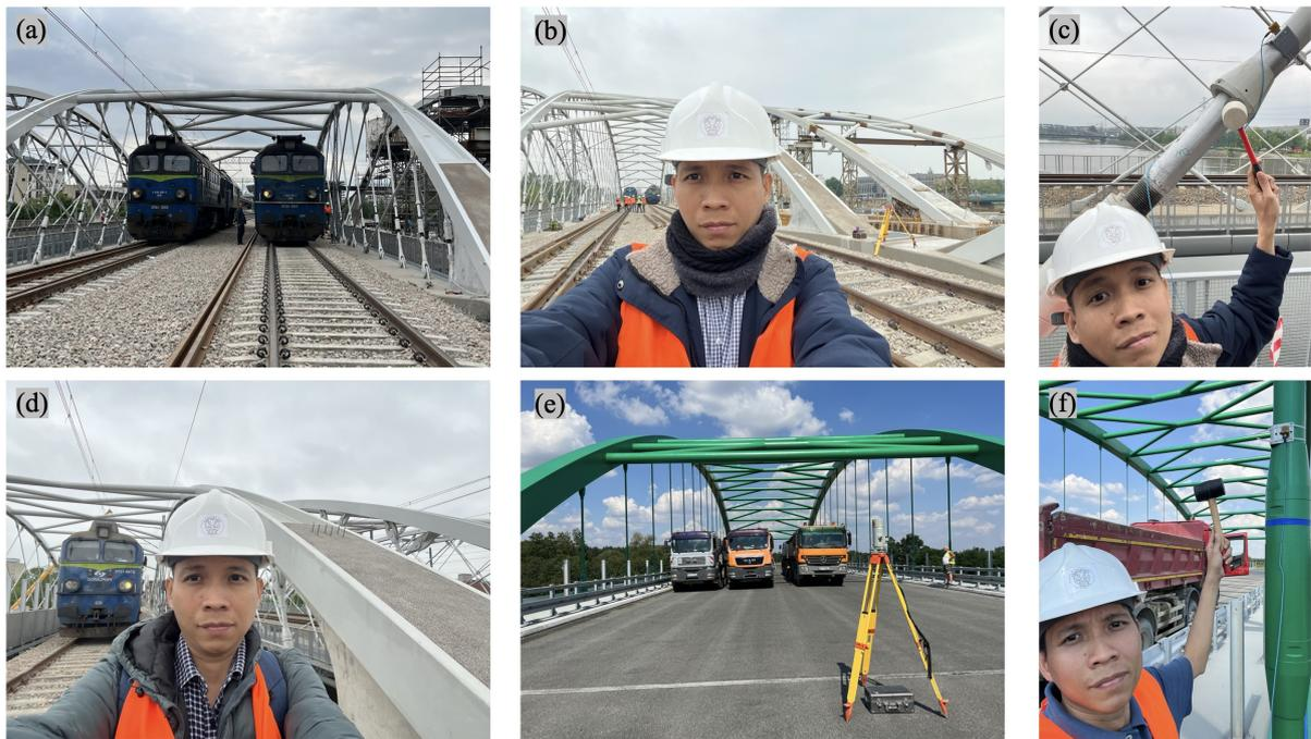
Figure 3.2: Diagnostic load testing for steel arch bridges: a), b), c), d) Vistula railway steel arch bridge in Kraków city; e), f) Steel arch bridge on the Kędzierzyn-Koźle (DK40).
