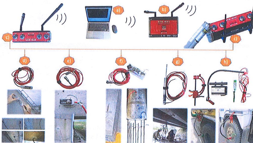
Fig. 5. The wireless structural testing system (STS-WiFi) for diagnostic load testing of existing bridge structures.
