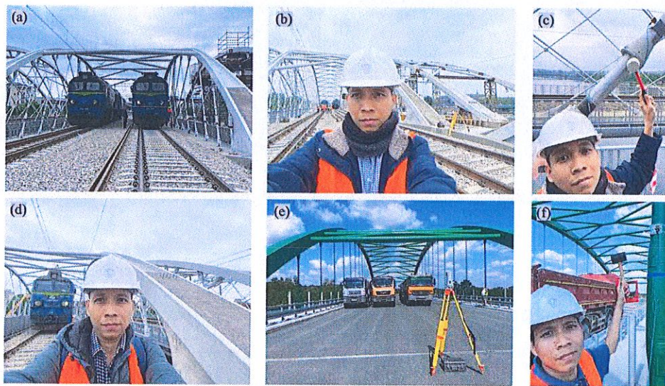
Fig. 4. Diagnostic load testing for steel arch bridges: a), b), c), d) Vistula railway steel arch bridge in Kraków city; e), f) Steel arch bridge on the Kędzierzyn-Koźle (DK40).
