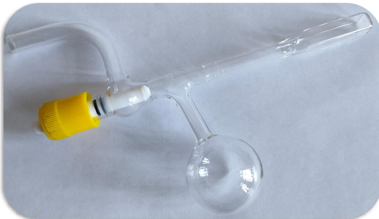
Figure 22. Special quartz cuvette for solution degassing used in photoluminescence studies in solutions.
