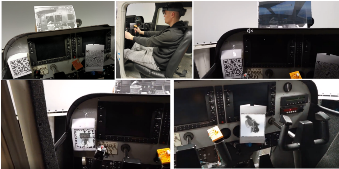
FIGURE 4.8: Various stages of augmented reality marker integration in flight simulator training, showcasing different marker placements and sizes for enhanced cockpit interaction and tracking accuracy.
