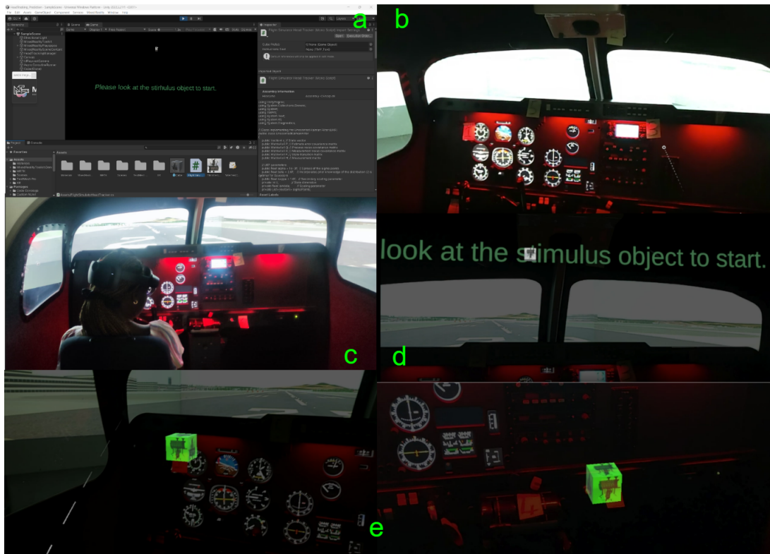
FIGURE 6.2: Experimental Setup and Cockpit Instrumentation. The figure shows the flight simulator setup used for head-tracking studies. Panels (a-b) display the pilot's view and calibrated cockpit, (c) the subject interacting with the cockpit, and (d-e) the visual stimuli and response interface. This setup enables precise tracking and analysis of head movements in response to simulated flight conditions.
