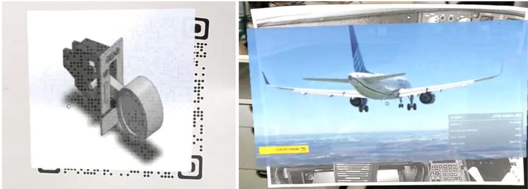
FIGURE 2.4: The left image shows the fiducial marker used to align the virtual cockpit instrument, and the right image shows a screen playing a video of a landing manoeuvre over a customized marker.
