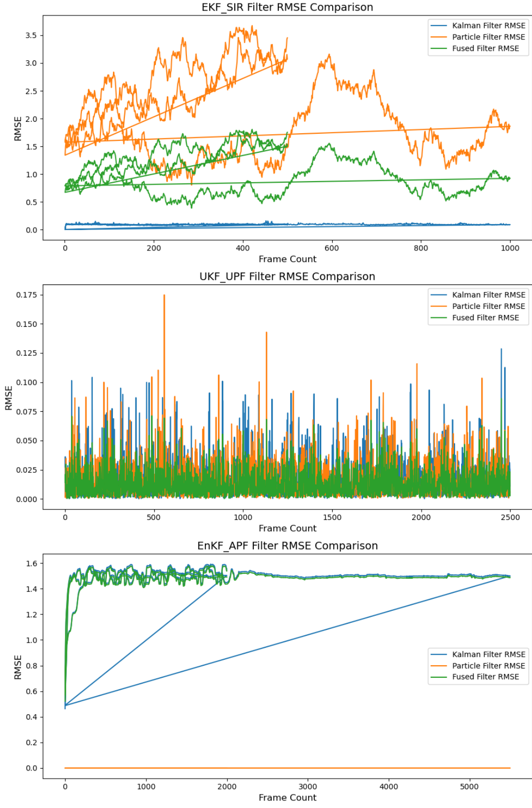
FIGURE 6.13: Comparison of RMSE values for Kalman, Particle, and Fused Filters across three datasets: EKF_SIR, UKF_UPF, and EnKF_APF, showcasing their performance and accuracy over increasing frame counts.
