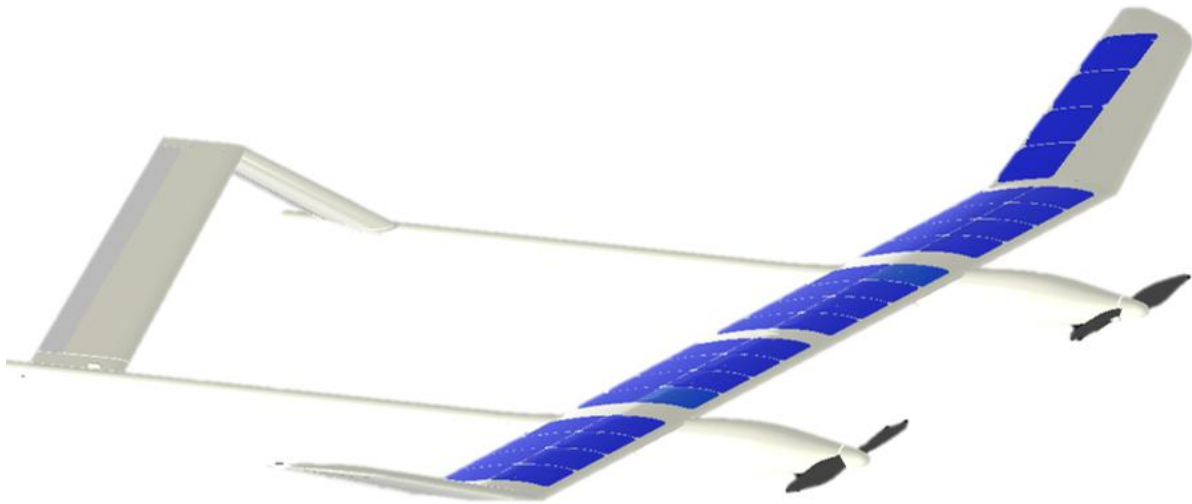
Fig. 114 Optimal tail configuration in case of stability criteria
