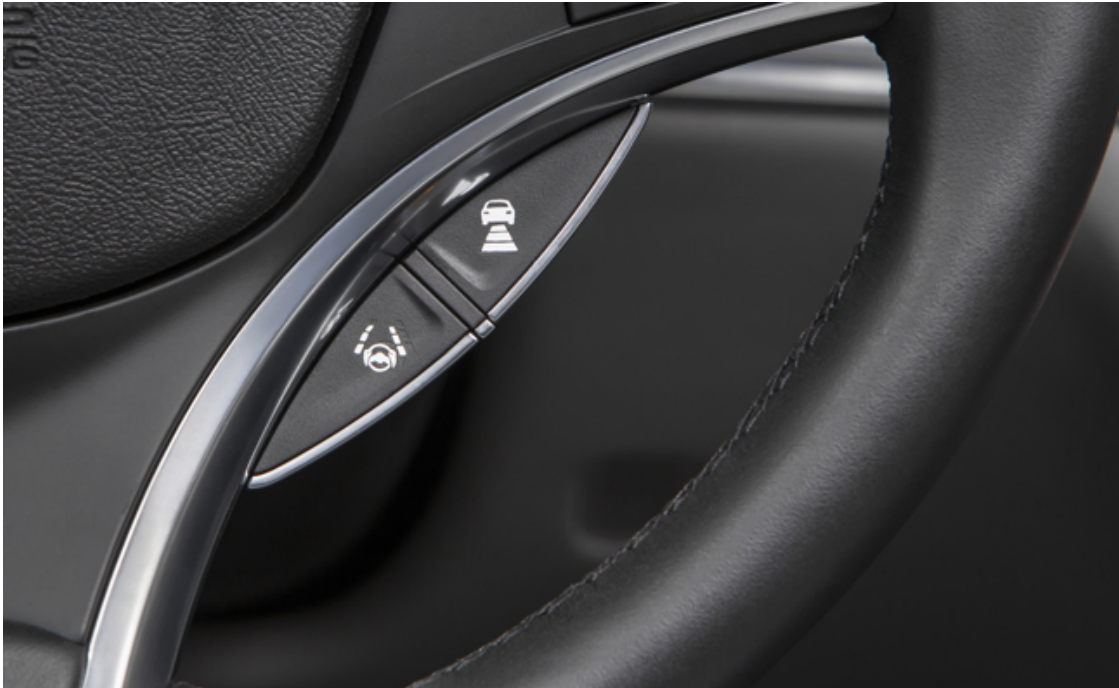
Figure 2.4: Acura’s MDX steering wheel buttons for enabling and disabling the LKA and ACC functions Image source: www.autoguide.com
