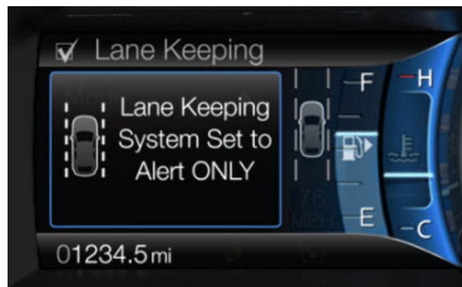
Figure 2.3: Ford graphical user interface showing that lane keeping system works in alert mode only. Image source: www.autoguide.com
