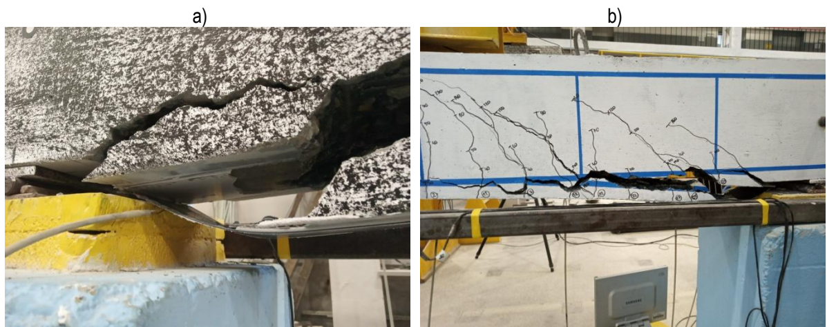
Fig. 4.12.: Typical failure mode (CSS) of beam specimens in series B (here B3b)
