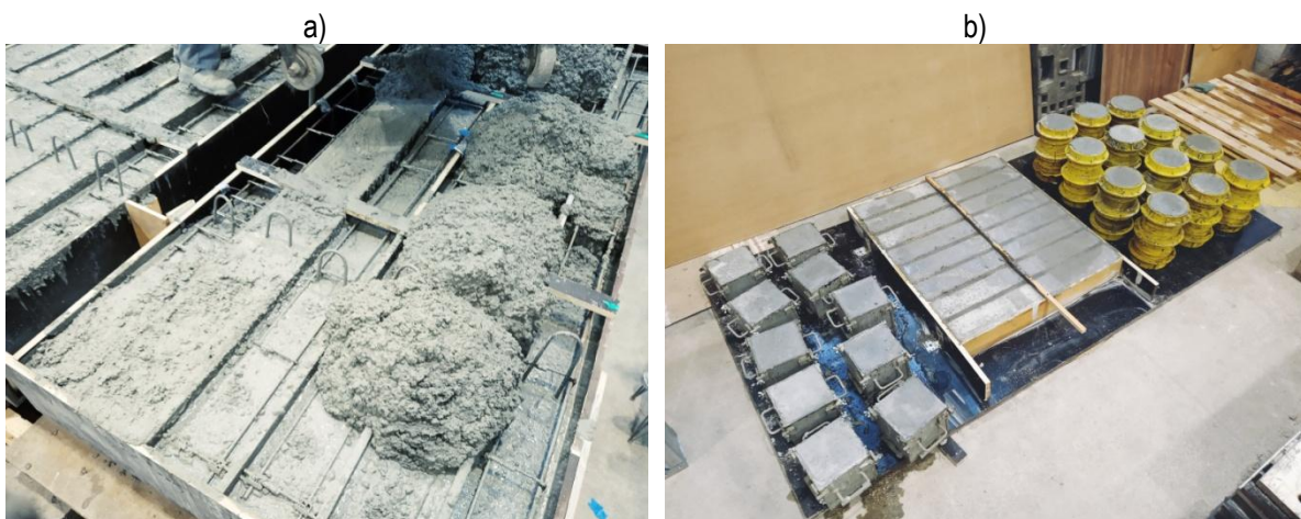
Fig. 4.5 a) Concrete pouring b) Concrete cubic and cylindrical specimens
