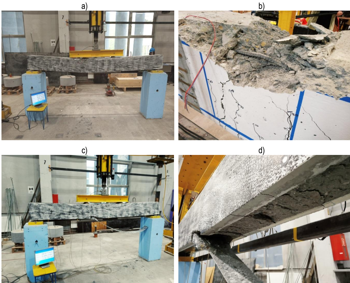
Fig. 4.10.: Typical failure mode of reference beam specimens A1 a) and b) and A2 c) and d)
