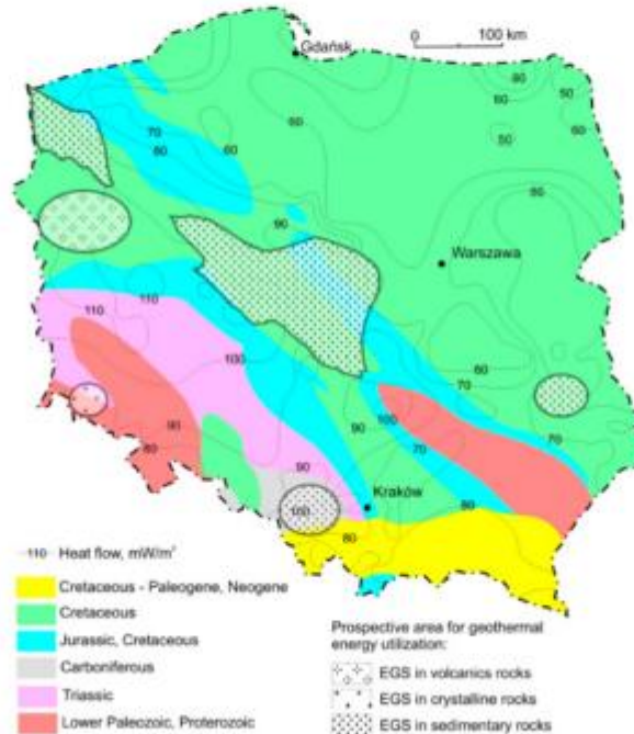
Figure 7. Prospective areas for conventional and unconventional geothermal energy utilization and Earth's heat flow density in Poland against the background of simplified geologic setting (based on [31,61,64]).
