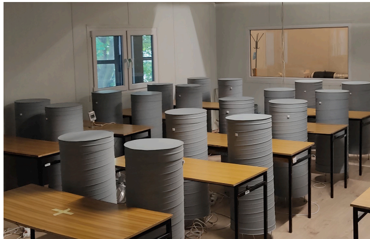
Fig. 1. Photo of the test room with desks and heated dummies.
