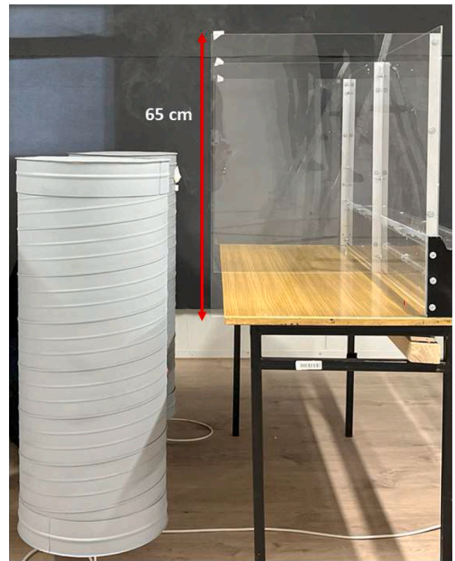
Fig. 1. Photo of designed partitions and two dummies at a desk.
