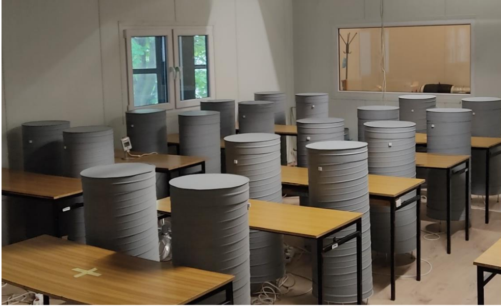
Fig. 6. Photo of the test room with desks and heated dummies.
