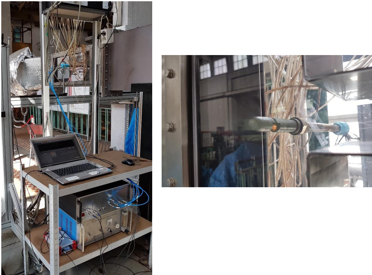
Fig. 2.7. View of the X probe measurement system during tests in the steam tunnel
