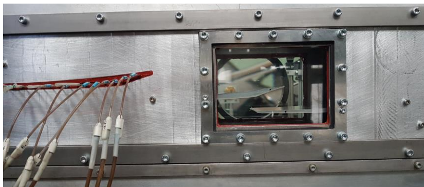
Fig. 2.4. Rotor blade cascade in the SUT test rig and the measuring equipment.
