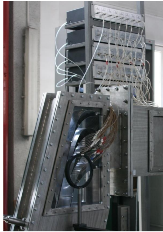
Fig. 2.3. Stator blade cascade in the SUT test rig and the measuring equipment.
