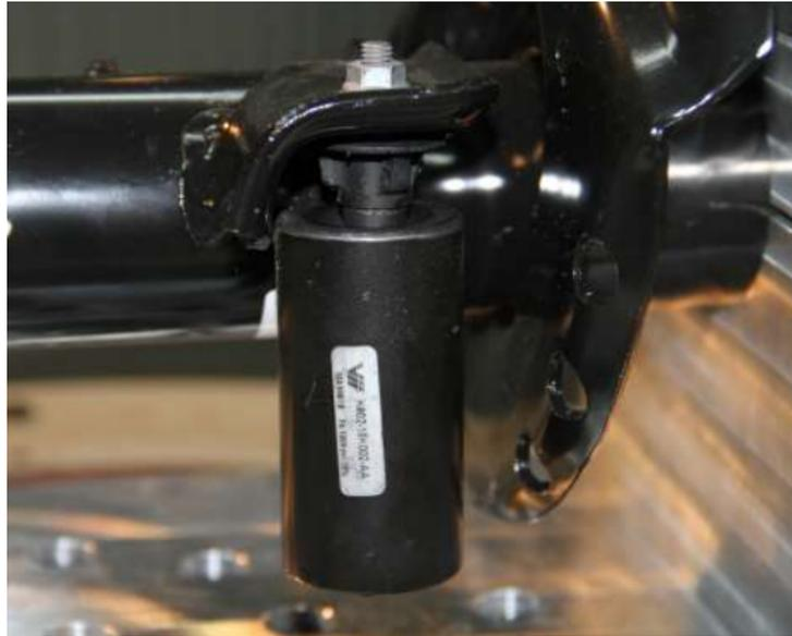
Figure 2.11: Exemplary design of mass absorber used to alter dynamic properties of the shock absorber structure (source: Courtesy of Tenneco Automotive Eastern Europe Sp. z o.o.)
