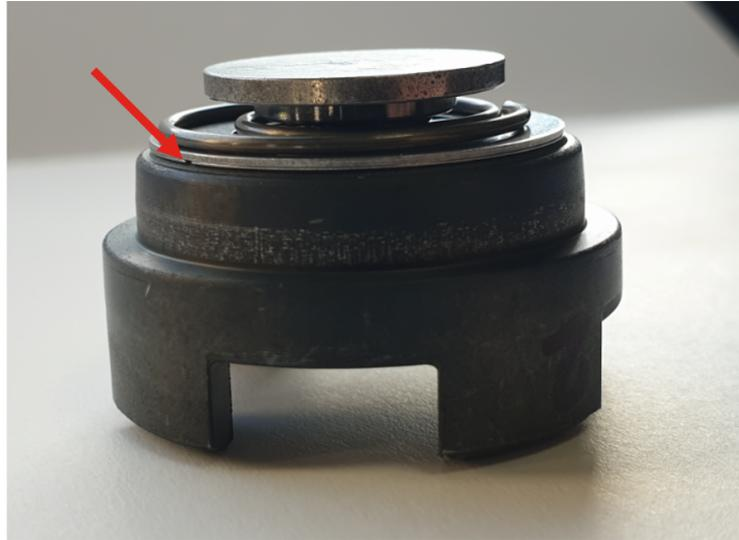
Figure 4.3: View of the purposefully introduced slot that influences the low flow rate part of the P/Q curve (valve bleed)
