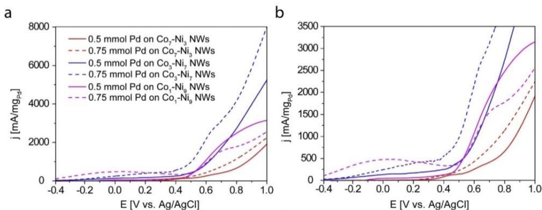
Fig. 10. (a) Comparison of the cyclic voltammograms of electrocatalysts in the form of cobalt-nickel nanowires with different Co:Ni ratios decorated by Pd in argon-saturated 1.0 M NaOH + 0.5 M CH<sub>3</sub>CH<sub>2</sub>OH solution at a scan rate of 20 mV/s; (b) plot showing an enlargement of the data between 0 and 3500 mA/mg<sub>Pd</sub>. Reproduced and modified with permission from <sup>10</sup>. Copyright (2022) Elsevier.
