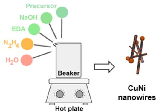
Fig. 4. Scheme of the synthesis procedure. Reproduced with permission from <sup>6</sup>. Copyright (2020) Springer Nature.
