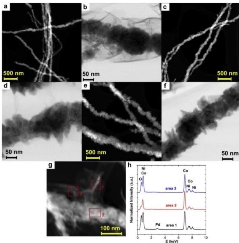
Fig. 9. STEM (a-g) images of CoNi NWs; h – EDX spectra of selected sample. Reproduced with permission from <sup>10</sup>. Copyright (2022) Elsevier.
