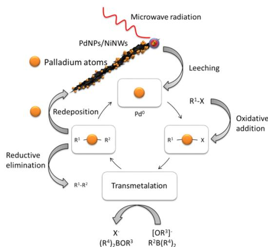
Fig. 7. Proposed mechanism for the PdNPs/NiNWs-catalyzed Suzuki cross-coupling reaction. Reproduced with permission from <sup>7</sup>. Copyright (2023) Elsevier.
