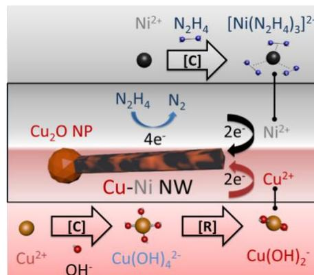
Fig. 5. Growth of a CuNi NW. [C] complexation, [R] reduction. Reproduced with permission from <sup>6</sup>. Copyright (2020) Springer Nature.
