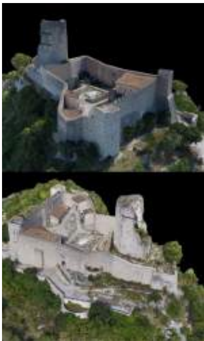
Fig.11 Rocca's point cloud processed in Recap Pro software (Elaborated in collaboration with Pelliccio A., Saccucci M.)
