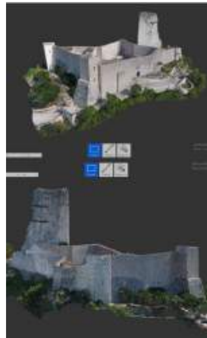
Fig.10 Textured model of the Rocca: different views of the point cloud processed in Recap Pro software (Elaborated in collaboration with Pelliccio A., Saccucci M.)
