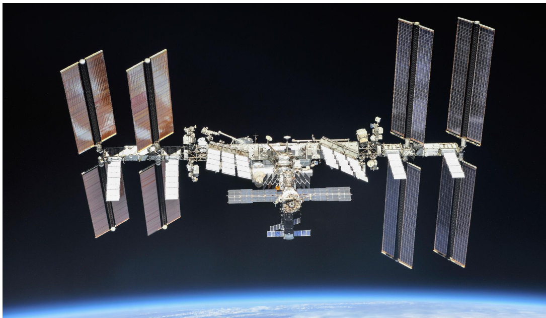
Fig. 53. International Space Station (ISS) in its full orbital configuration, including the U.S. and Russian segments, truss structure with photovoltaic arrays, laboratory modules, life support systems, and robotic elements. (source: NASA – ISS, n.d.).
