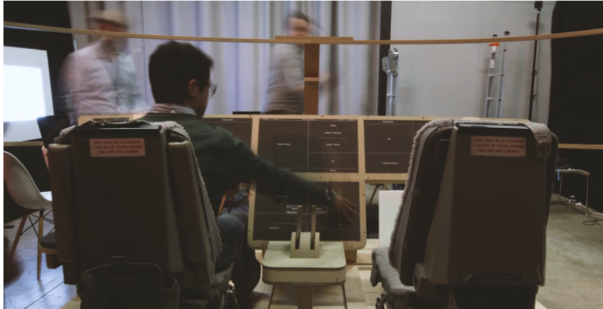
Figure 3.2: Future System Simulator’s MDF flight deck prototype. Reproduced under the courtesy of DCA Design International [97].
