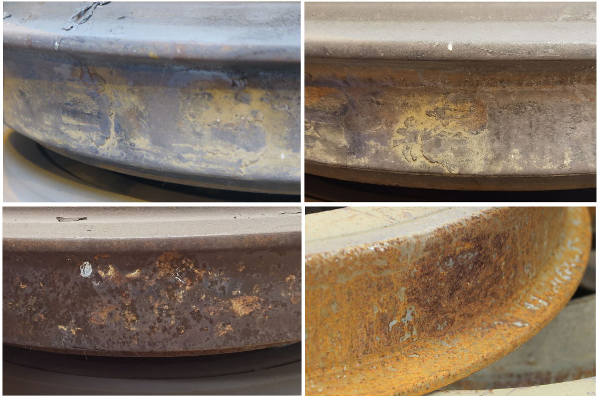
Figure 1.1: Typical wheel defects captured from a tram depot
